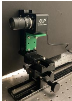
Figure 2. A camera array with a translation stage and 3D printed holder in the lab environment.
