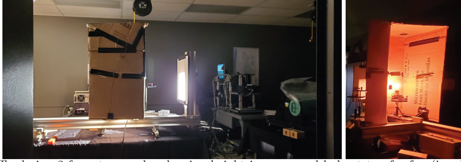
Figure 9: Baffle design 2 from two angles showing height increase and hole at top for fan (i.e., heat removal).
