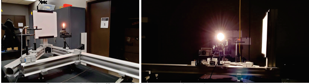
Figure 21: Set up with no baffle. Both the sensor and FEL lamp are in the open air.
