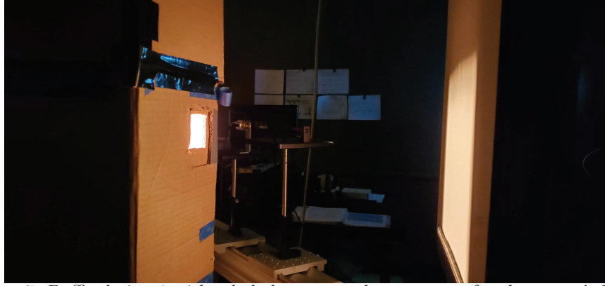
Figure 7: Baffle design 1 with a hole large enough to account for the sensor's FOV.
