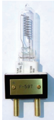
Figure 1: Typical 1000W FEL lamp used for spectral calibration.
