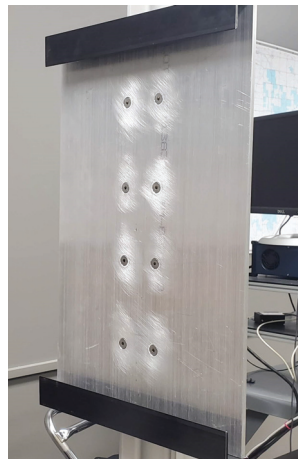
Figure 6: Lambertian plaque holder.
