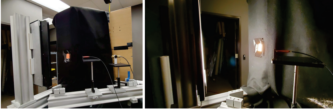
Figure 18: Set up for baffle covered with black felt.
