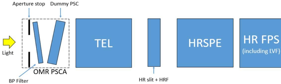
Figure 1-3 Scheme of the subsystems inside the FLORIS OMR
