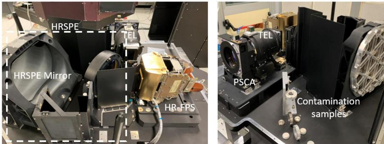
Figure 1-4 OMR model internal layout
