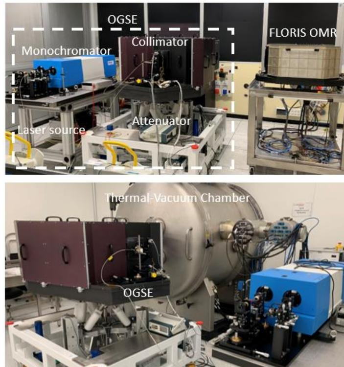
Figure 2-2 FLORIS OMR SPST measurement setup for 'in-air' measurement (top panel) and for the vacuum measurement (bottom panel) where the OMR is inside the TVC
