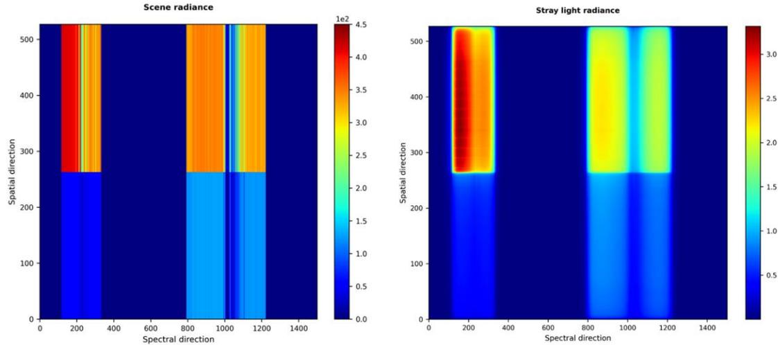
Figure 4-1 Reference scene radiance (mW/m<sup>2</sup>/sr/nm) (left) and corresponding L0 (without correction) SL radiance (right). The upper part of the figures represents the TOC cloud radiances while the lower part represents the reference vegetation radiances.
