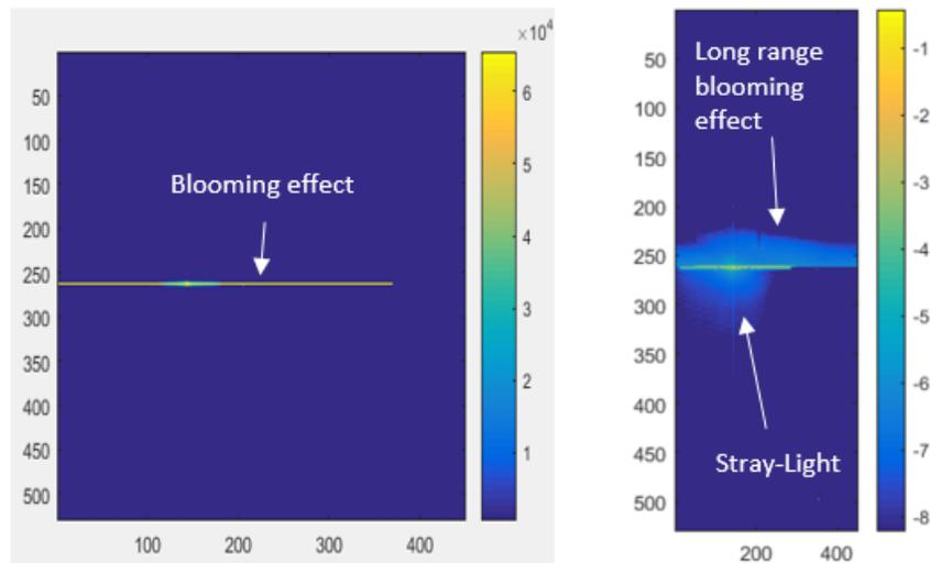
Figure 2-3 – Left: density plot (linear scale) of an high flux acquisition on HR2 detector, the blooming produces a stripe in the spectral direction. Right: Example of in field, in band SPST map (logarithmic scale) with nominal voltage configuration. Long range blooming effect overcomes SL signal in the illuminated top half.
