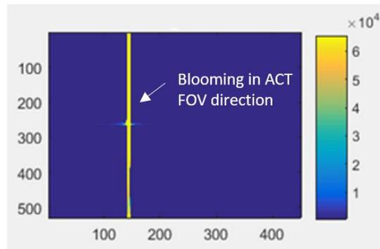
Figure 2-4 – High flux measurement with modified clock high voltage. The blooming preferential direction turns from horizontal (spectrum) to vertical (FOV ACT).
