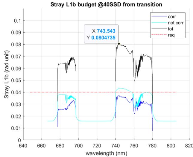
Figure 4-3 L1b (after correction) SL level at 40 SSD from the transition between a bright and a black scene.
