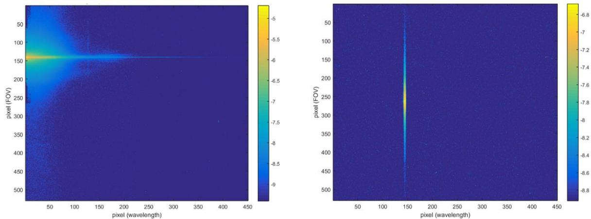
Figure 3-1 Left: Example of OOB measured SPST map, 9-10 orders of magnitude have been reached. Right: Example of OOF SPST map. The illuminated spot is blocked by the slit chip and the SL generated by fore-optics is visible through the slit aperture.
