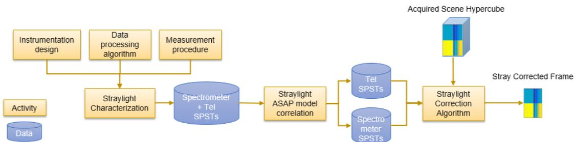
Figure 1-2 Scheme of the FLORIS SL correction process
