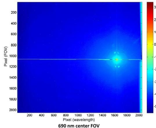
Figure 2-1 SPST map acquired during the FLORIS breadboard campaign [8]. The primary spot is at 690 nm wavelength and axial FOV, the intensity is in logarithmic scale. The four triangular feature are due to the not optimized grating used for the breadboard. The horizontal dark line is due to the blooming of the service detector while the bright vertical feature on the right part is due to the service camera read-out register.
