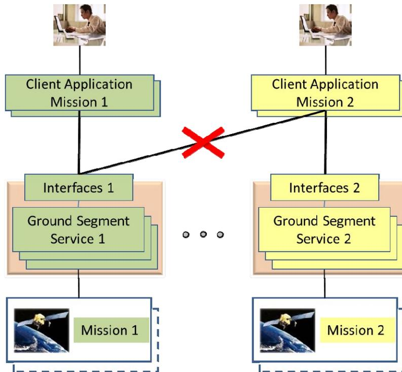
**Figure 4-2: Access to EO Mission Products through Ground Segment Services**
