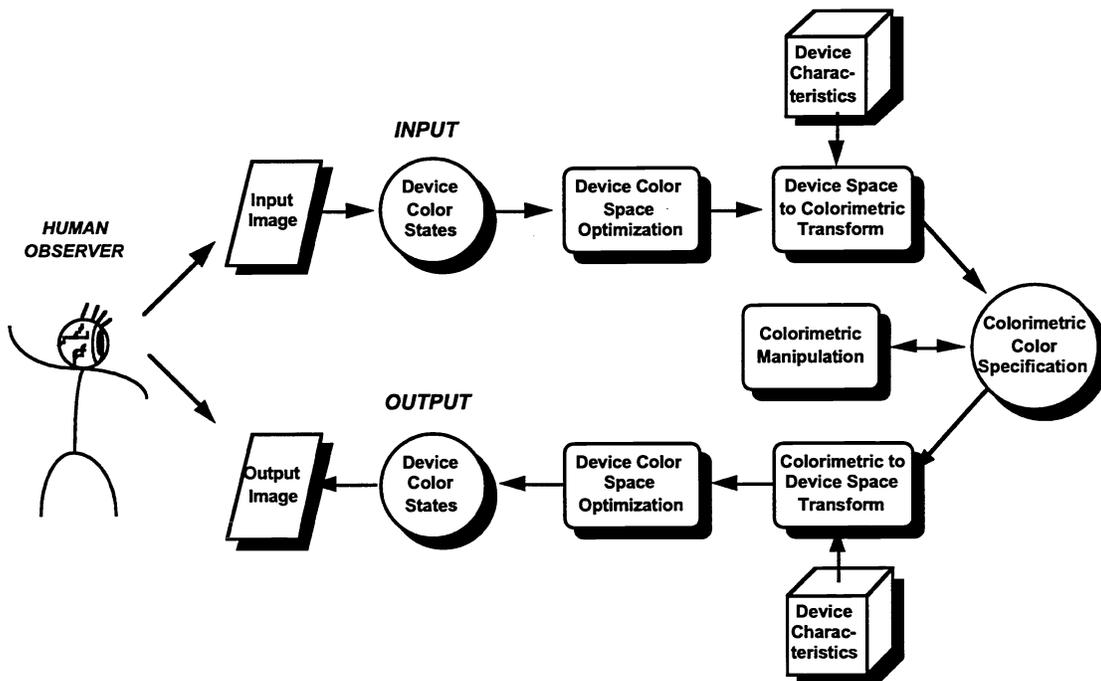
Figure 1 - The device independent imaging pipeline
