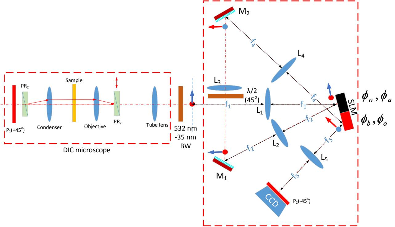
Figure 1. Proposed optical setup for the QDIC module
