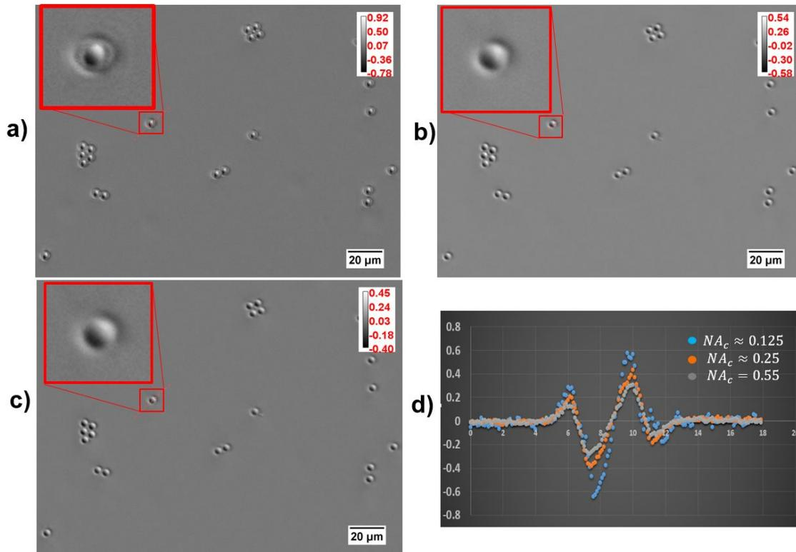
Figure 2. a - c) Quantitative phase difference images of 3-micron polystyrene beads in dry air at different values of  $NA_c$ . d) Cross-section values along the line profiles specified in a-c).
