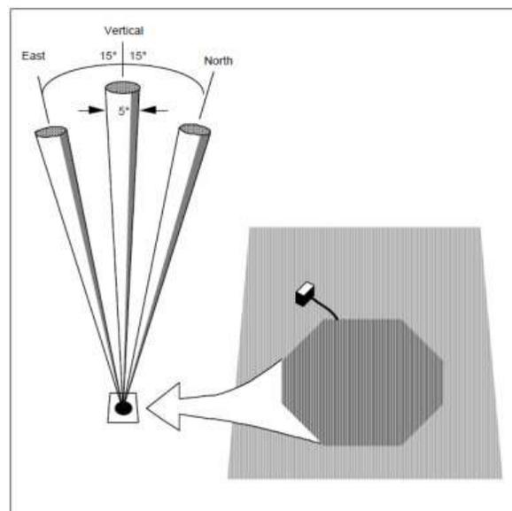
Figure 11. A schematic of the DRWP's beam configuration<sup>12</sup>.
