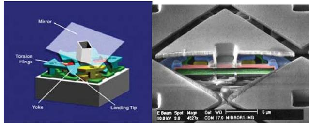
Figure 9. Texas Instruments' DMD: Principle and SEM photograph, courtesy Texas Instrument
