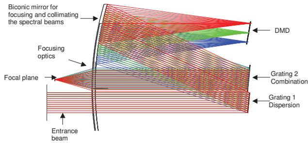
Figure 11. Optical MEMS based spectrometer
