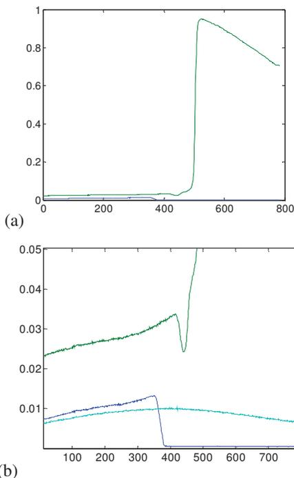
Figure 7. Cloud removal experiment; a) profile of the FOV including the scene (left part) and the clouds (right part) when the programmable slit is all ON (green curve) and when the micro-mirrors located on the bright area are switched OFF (blue curve); b) Close-up view of the transition area; the light blue curve represents the perfect scene, without clouds.
