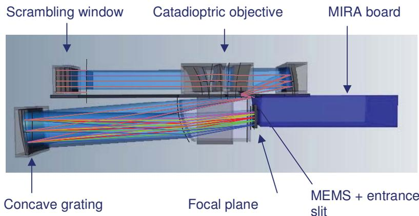
Figure 6. Superimposition of the optical design and of the CAD view
