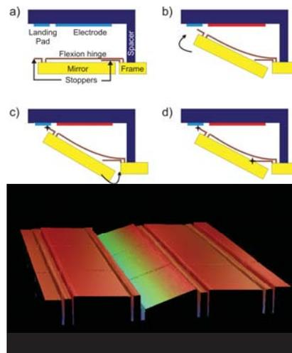
Figure 1. Micro-mirror for multi-object spectroscopy:
