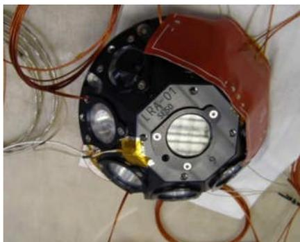
Figure 4. LRA equipped with its heater.
