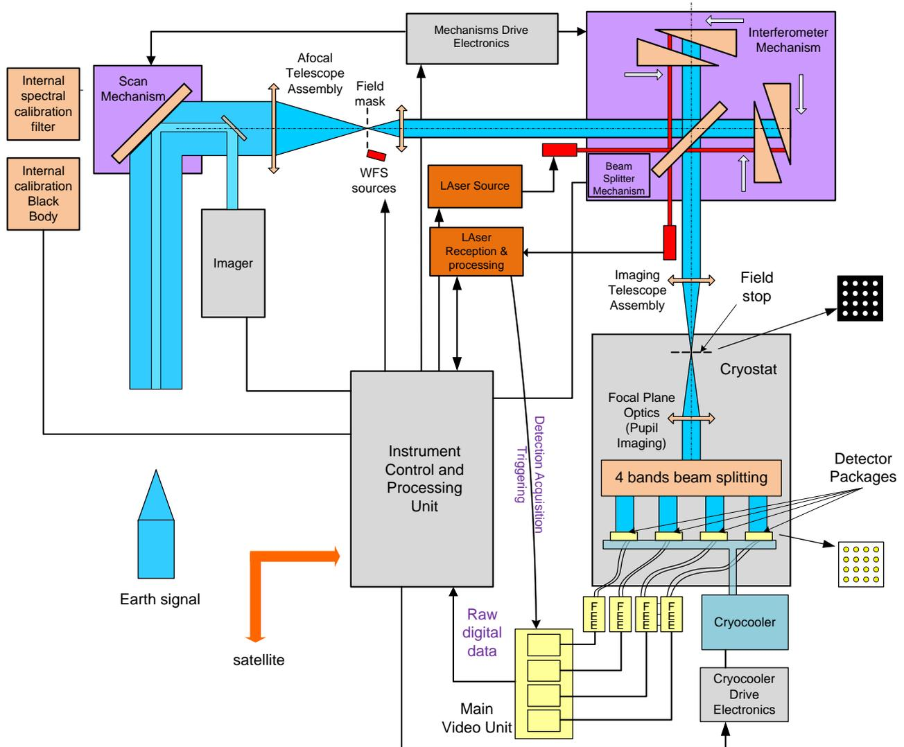
Figure 1. block diagramme of the IASI-NG instrument
