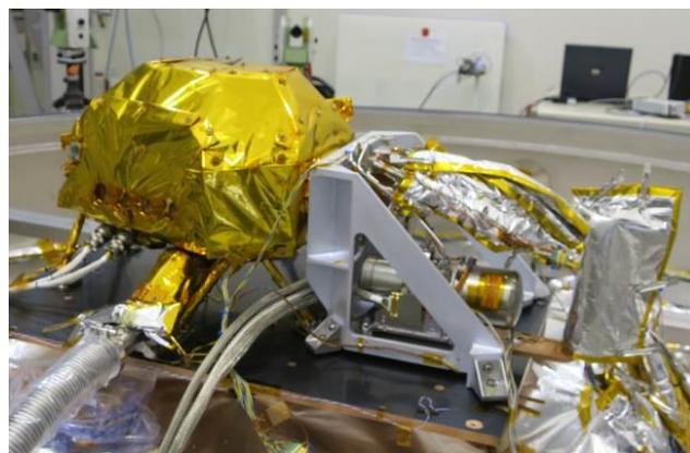
Figure 6. IASI-NG cryostat during vibration test and prior to thermal vacuum test
