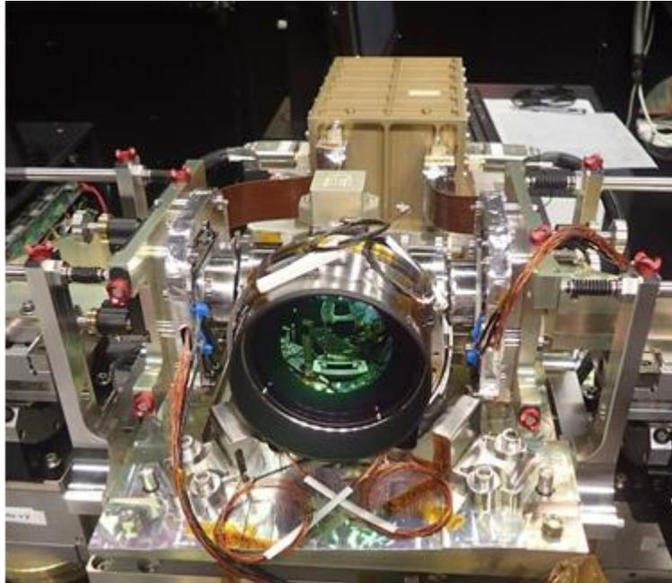
Figure 7. Alignment of the micro-bolometer detectors on the optics of the Imager
