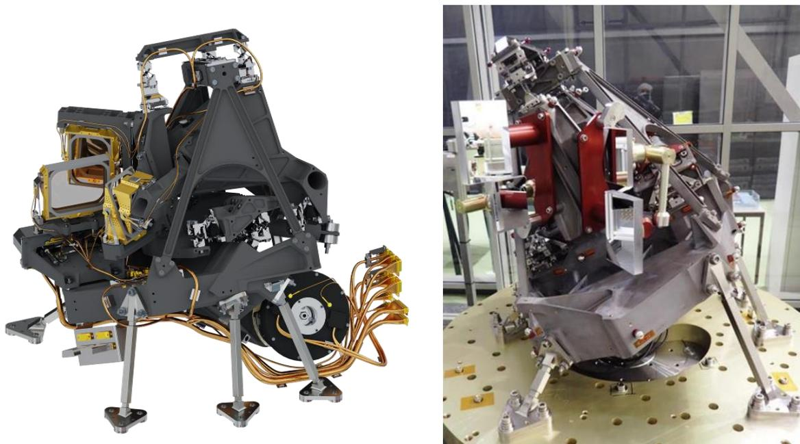
Figure 4. CAD model and actual IASI-NG interferometer mechanism
