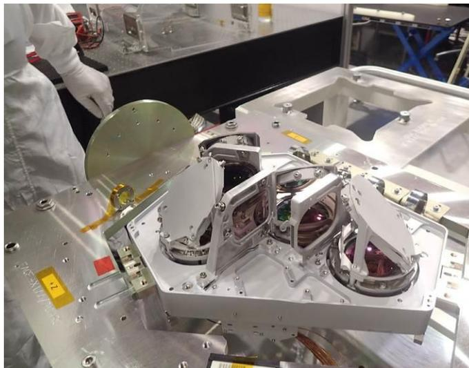
Figure 5. folding mirrors and dichroic plates on the cold optical bench
