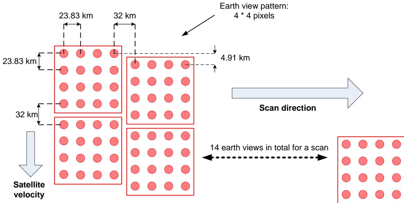
Figure 2. Instrument FOV footprint on ground and spatial sampling
