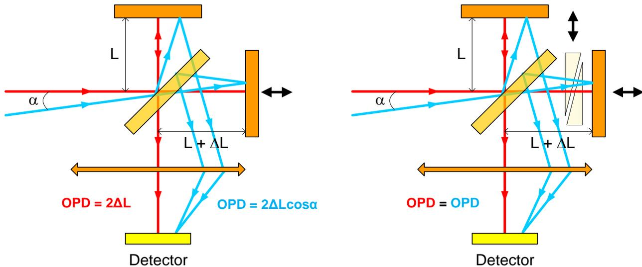
Figure 3. The OPD variation in the FOV is compensated for by a variable thickness KBr plate
