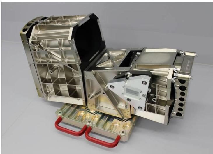
Figure 1. Optical system of the DESIS instrument. The telescope is on the left side, the spectrometer on the right. The light gray, triangular body is a detector dummy.
