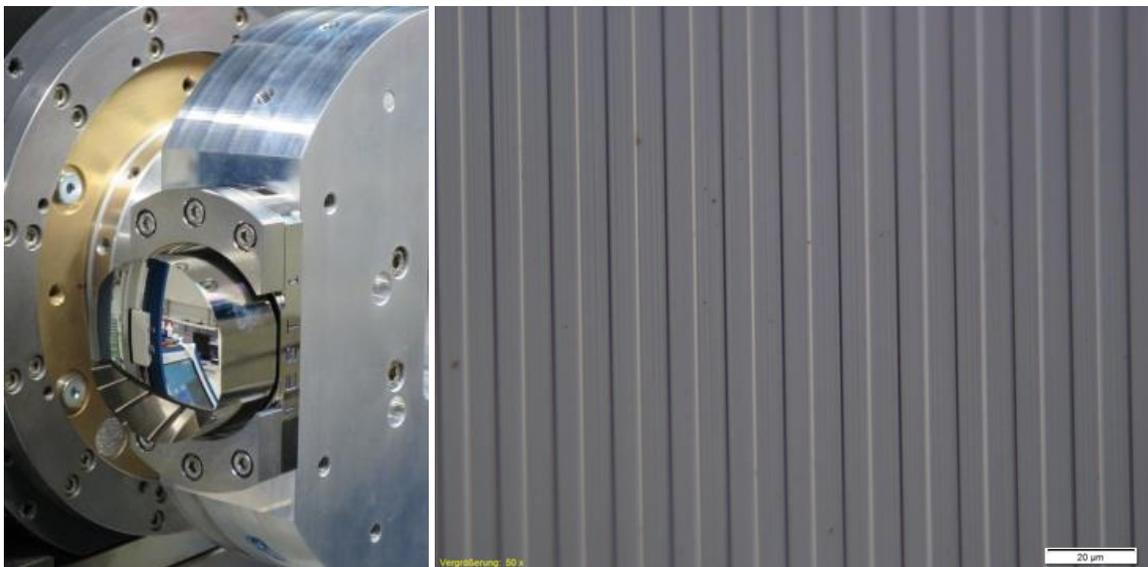
Figure 4. Manufacturing setup for the reflective grating (left) and microscopical image (right).
