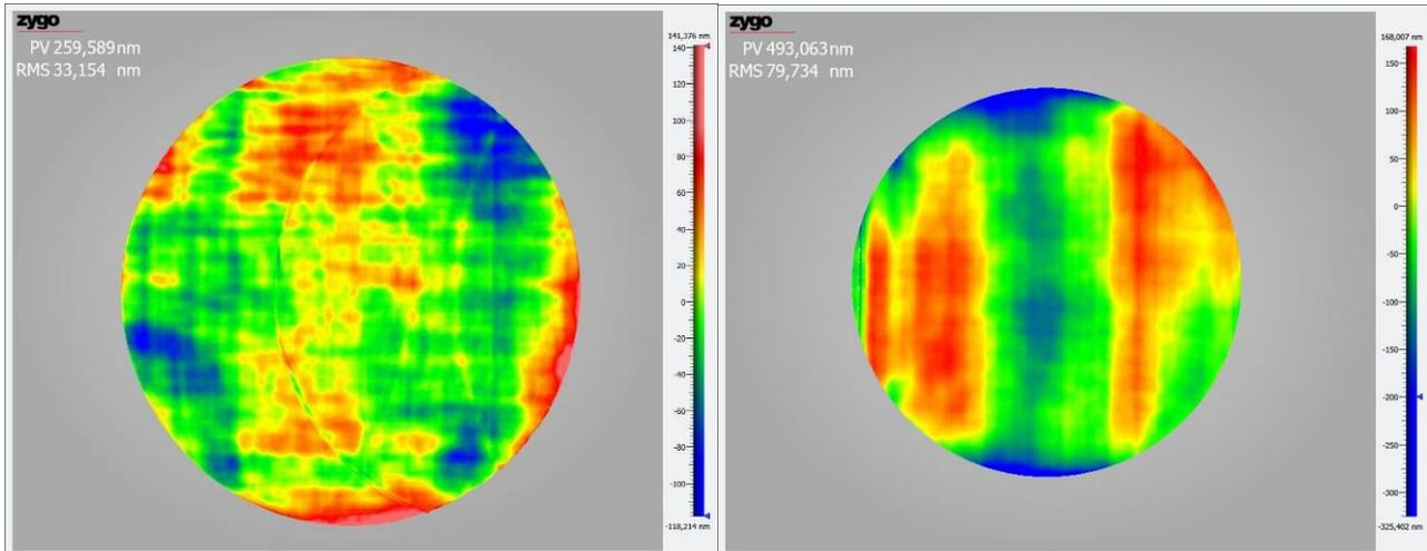
Figure 6. Measured wavefront errors of the TMA (left) and the spectrometer (right). The measurement position is in the center of the field of view.
