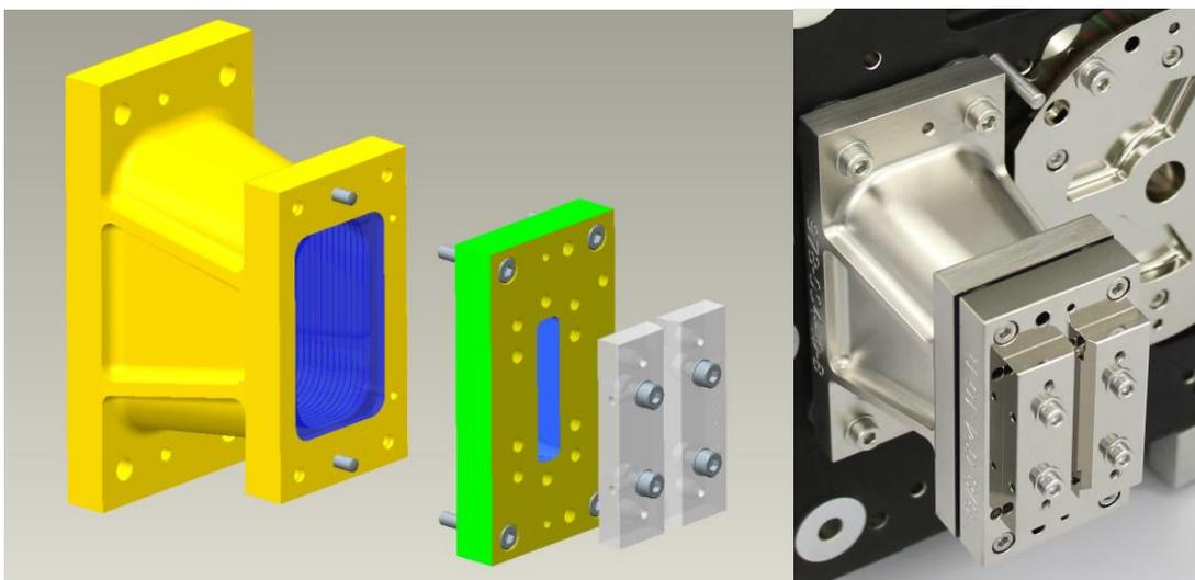
Figure 5. Exploded view (left) and image of the slit assembly mounted to the TMA (right).
