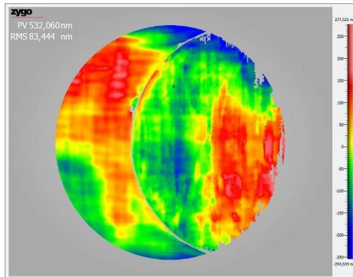
Figure 7. Measured wavefront errors of the complete optical system measured in the center of the field.
