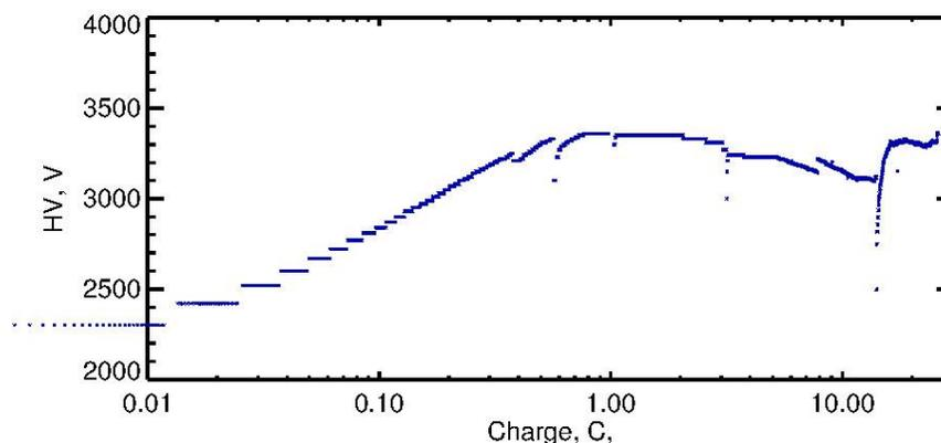
Figure 4. CEM HV as a function of the total accumulated charge while the CEM gain is constant. Taken for the room temperature.
