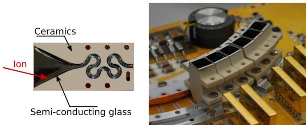
Figure 2. Left: Ceramic CEM design. Right: CEM array installed in PAS prototype.
