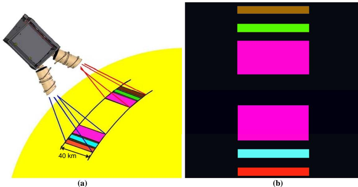
**Fig. 1.** In (a) STC Stereo concept. In (b) position and size of useful filter strips images on the detector area (in black). Note that not illuminated gaps are present between each filter image.
