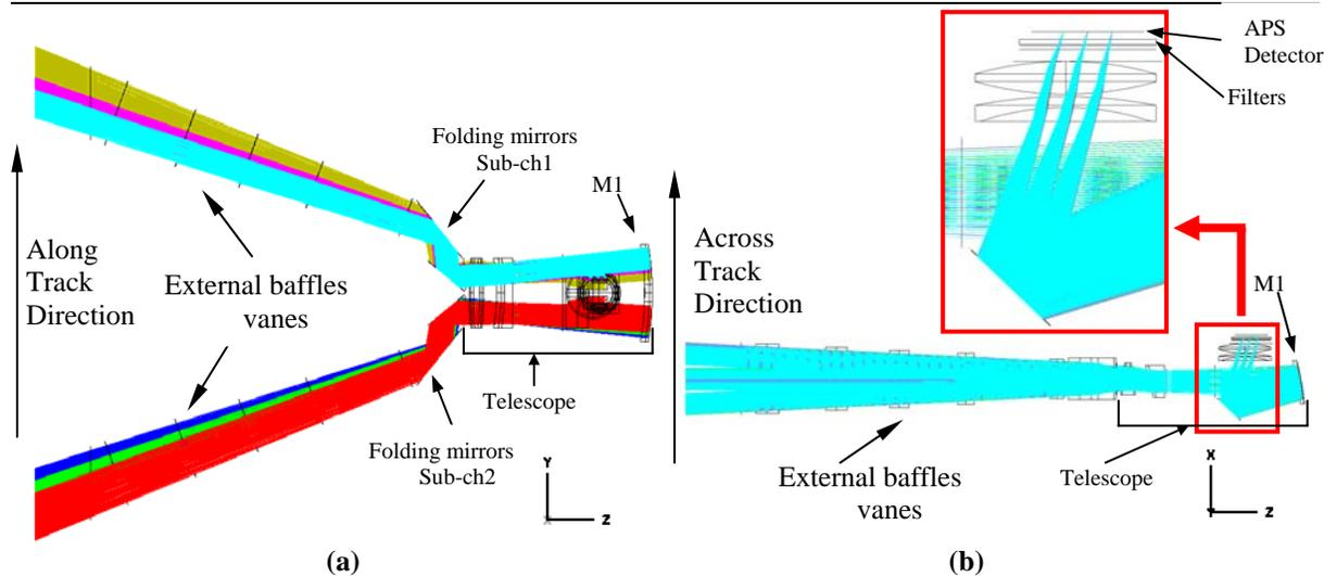
**Fig. 2.** Final overall STC optical layout. The whole STC optical design is shown: in (a) the configuration is viewed in the plane defined by the along track and nadir directions; in (b) the projection in the orthogonal plane, the one including across track and nadir directions, is given. In the inset, an enlarged view of the focal plane region helps to better follow the rays which are focalized on the APS detector.
