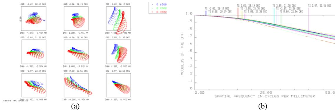
**Fig. 3.** STC optical performance: (a) spot diagrams; (b) MTF for the panchromatic filter.
