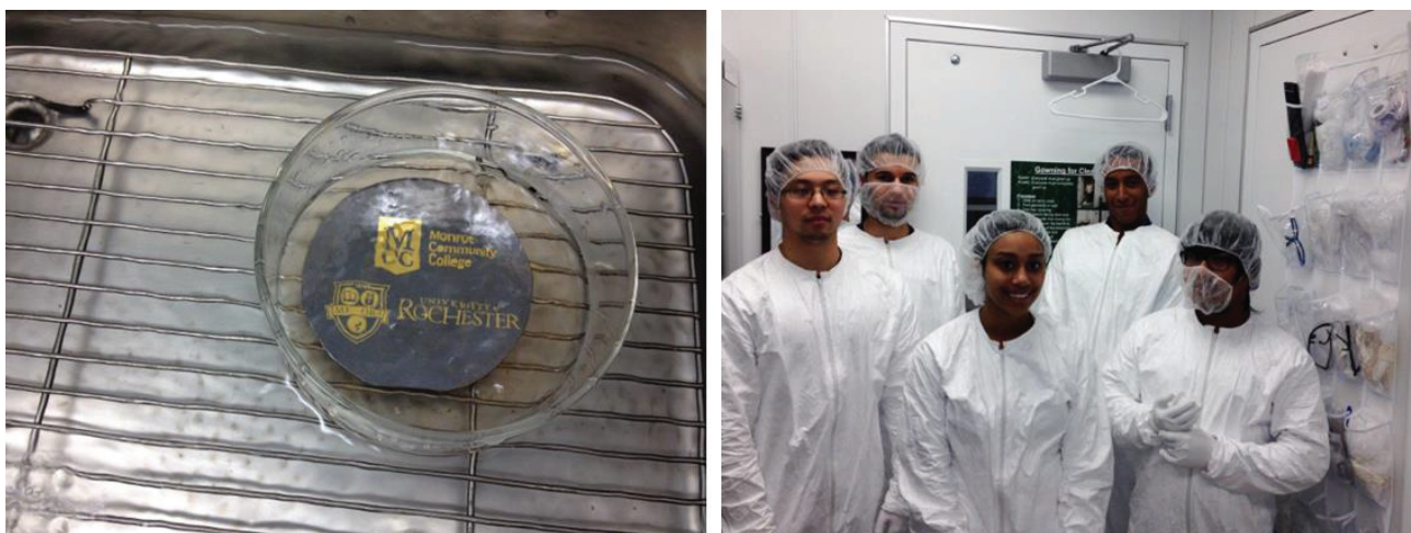
Figure 12. LEFT: MCC and UR logos prepared by MCC students using photolithography and vacuum deposition of a metal. RIGHT: One group of MCC students in the UR clean-room garments near the entrance to the clean room.
