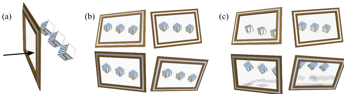
Figure 2. Light information of a Scene: (a) The direct view of the scene. (b) Rotation of a scene with only amplitude information. (c) Rotation of a scene with amplitude and phase information.
