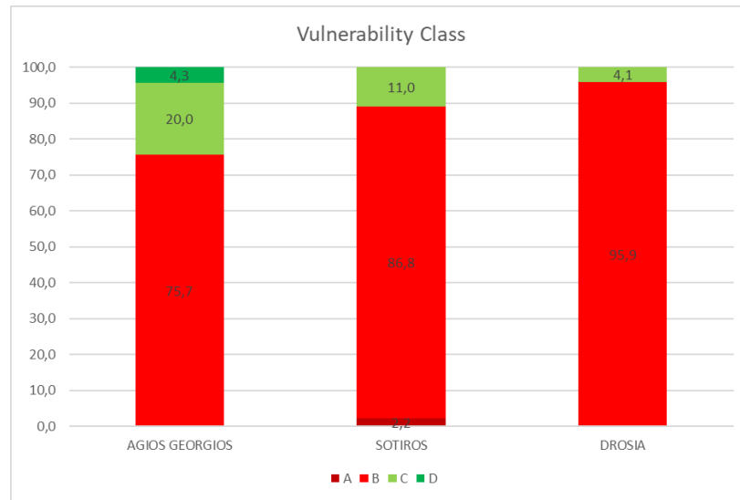
Figure 6 Investigated buildings distribution on the vulnerability classes
