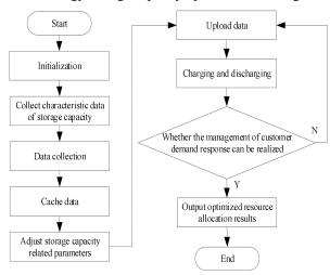
Figure 1. Flow Chart of Distributed Energy Storage Capacity Optimization Configuration
