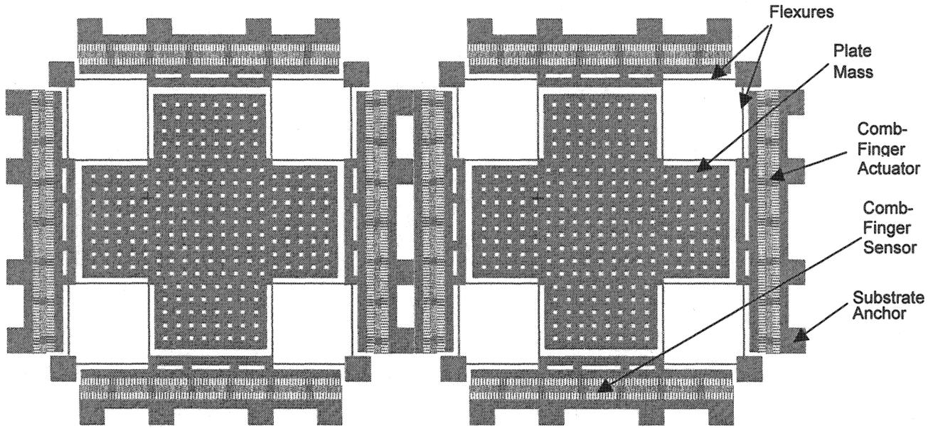
**Figure 1: AMCOM Developmental Roll Rate Sensor**
