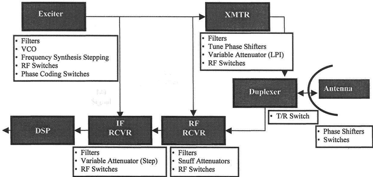
**Figure 7: RF Radar Block Diagram**
