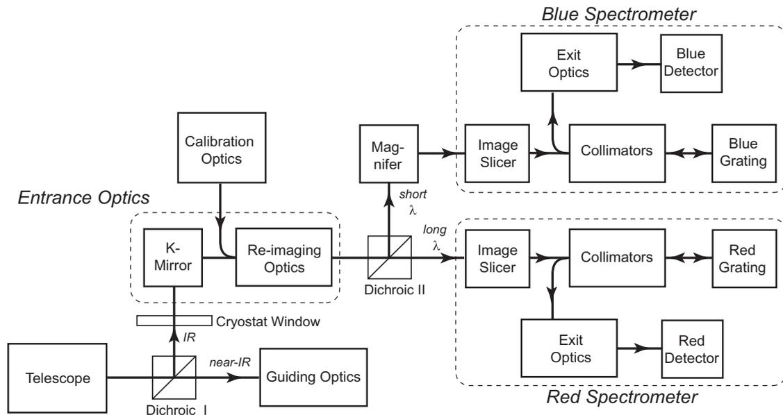
**Figure 2.** A simplified schematic overview of the FIFI LS optics. Calibration optics and intensity sources can be switched into the path via a flip-mirror to provide flat-fielding of the detector pixels.
