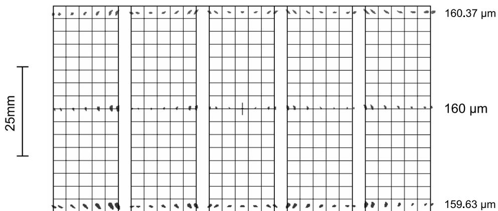
**Figure 6.** The final imaging of the dispersed beam at a wavelength of  $160 \mu\text{m}$  in the long wavelength channel.
