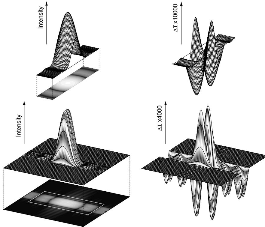
**Figure 9.** The diffraction effects on the slicer and capture mirrors calculated using the vectorial treatment on the left. On the right, the differences between two polarizations. The polarization difference on the top is most likely numerical rounding errors, and those on the bottom are real variations but insignificant.
