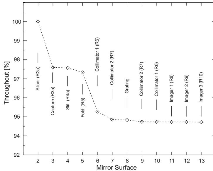
**Figure 10.** The light loss thru the optics due to pure diffraction and vignetting effects. Note that the largest losses are from the slicer system and the first Collimator mirrors.
