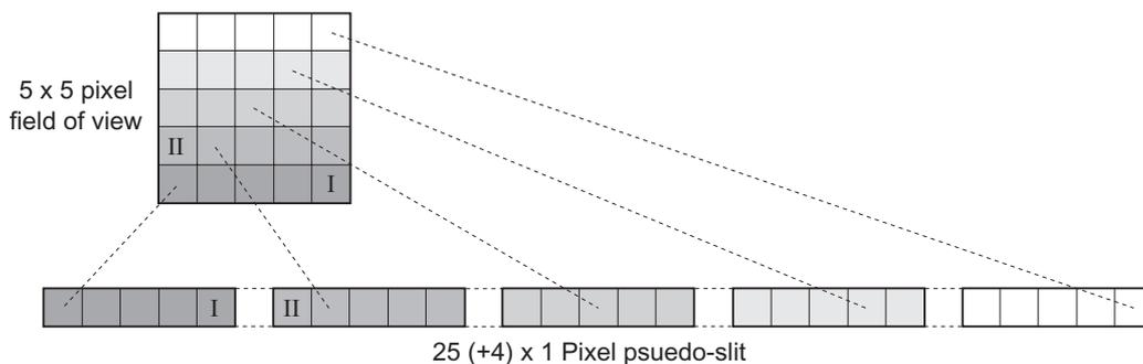
**Figure 1.** A detail showing the basic design premise for the FIFI LS image slicer. The optics must slice the rows of the 5 $\times$ 5 pixel field of view into a 25 $\times$ 1 pixel pseudo-slit. The gaps in the slit are added to reduce cross-talk between nonadjacent field pixels (e.g. pixels I and II).
