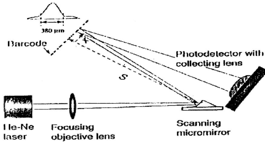
Fig. 7. Schematic of an Experimental Setup for Microscanner Characterization and Barcode Reading.
