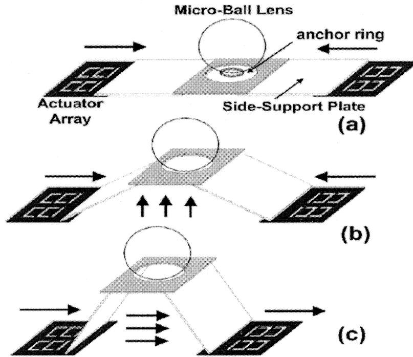
Fig. 3. Schematic of Micro-XYZ Stage Picking up and Moving an External Micro Ball Lens.
