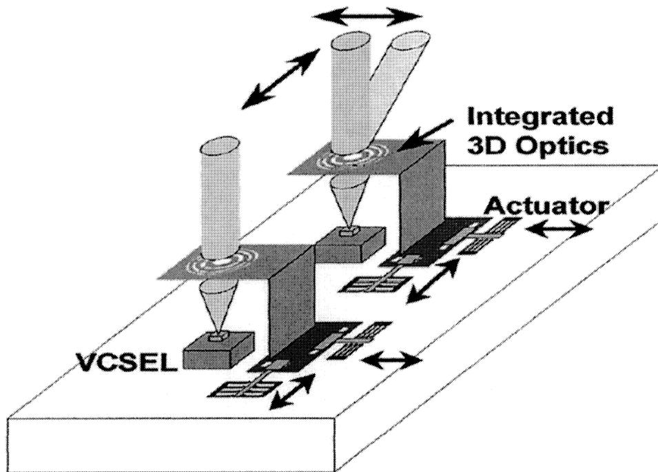
Fig. 4. Schematic of Scanning Microlens Integrated with Vertical Cavity Surface-Emitting Lasers.
