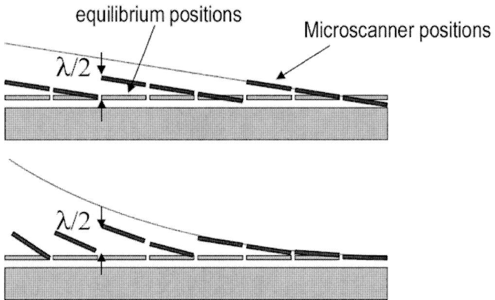
Fig. 5. Schematic Representation of the Operation of a Scanning Phased Array
