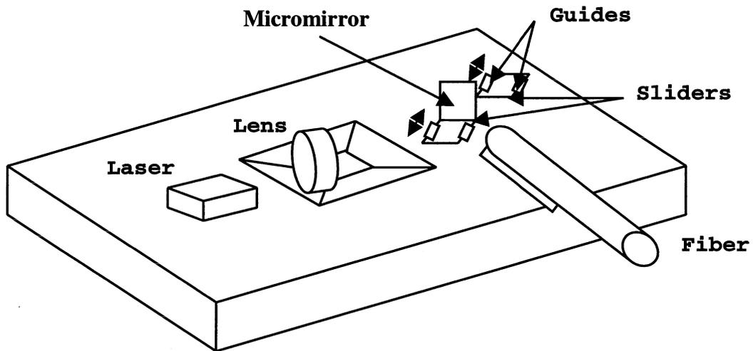
Fig. 6. Fiber-Coupled, Semiconductor Laser Module with On-Chip Alignment Mirror.
