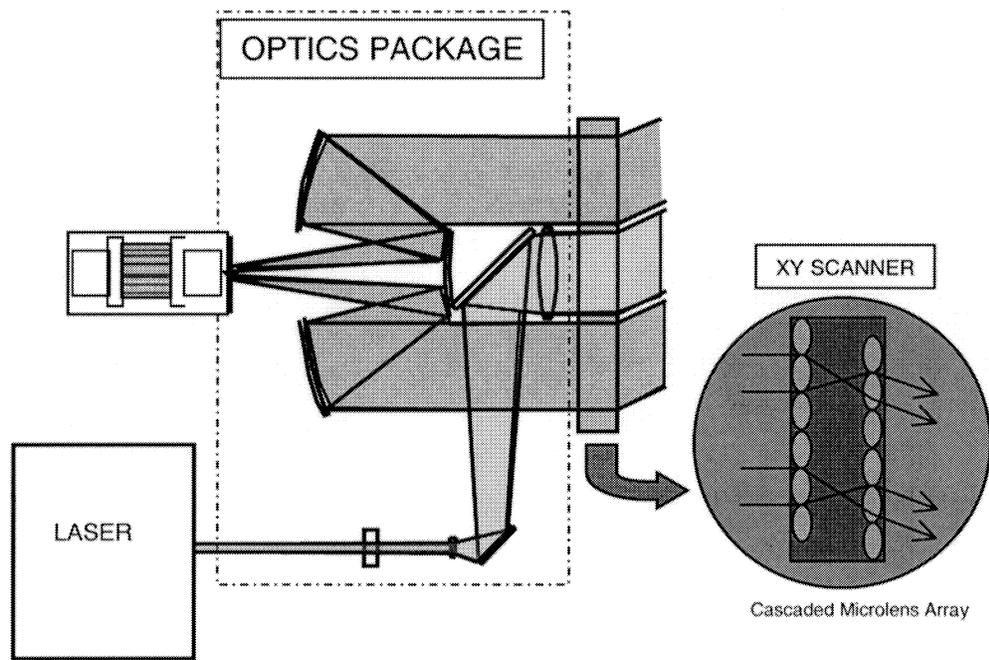
**Fig. 9. MEMS-Based Phased Array Scanner**
