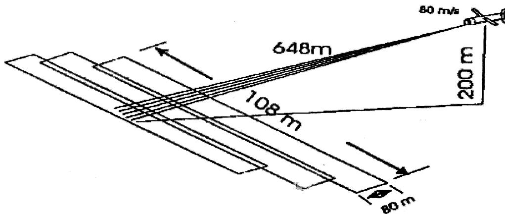
Fig. 2. LADAR Seeker Acquisition Scan Footprint.
