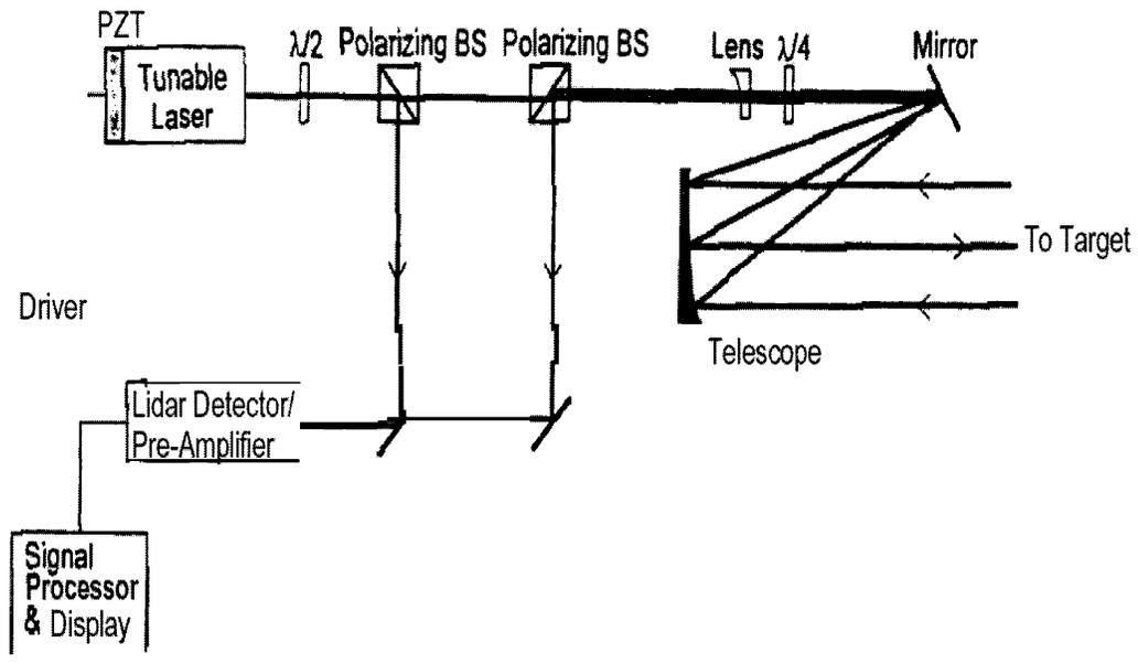
Fig. 8. Frequency-chirp Lidar Using A CW Tunable Laser
