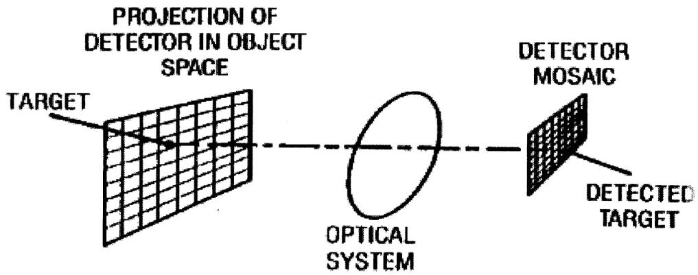
Fig. 1. Conceptual Diagram Illustrating the Basics of Focal Plane Array Imaging.
