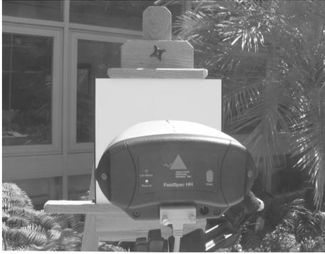
**Figure 6.** Radiance measurement using ASD FieldSpec Handheld spectroradiometer
