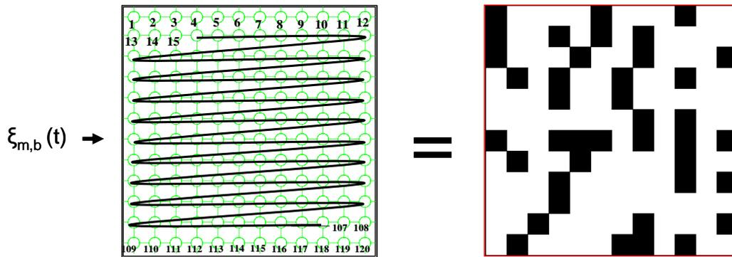
Fig. 5 EEG data segment stored as input on a two-dimensional CNN leading to an image with binary pattern
