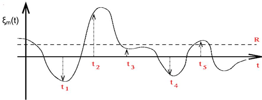
Fig. 3 Event of the pattern detection algorithm. While  $\xi_m(t)$  is below a certain level  $R$  at  $t_1, t_3$  and  $t_5$  it is above  $R$  at  $t_2$  and  $t_4$ .
