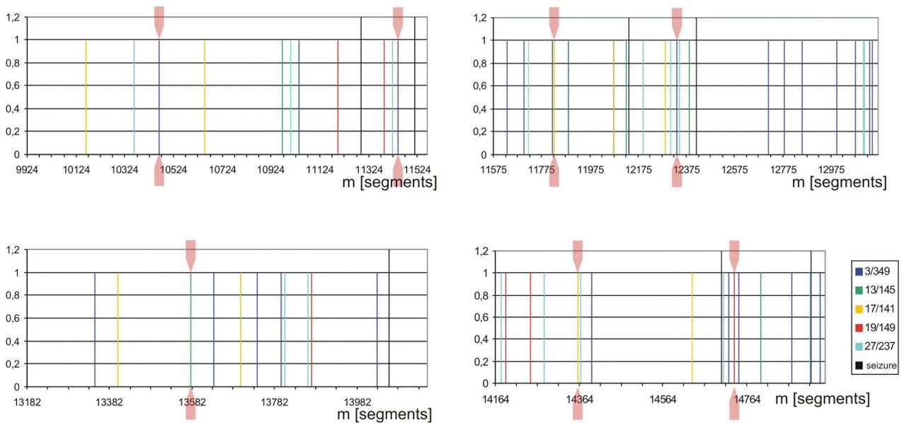
Fig. 14 : Results of the Pattern Detection Algorithm (PDP) based on five observed electrode points. Seizures are marked by black vertical lines, seizure warnings are marked by grey arrows. A seizure warning is given when the pattern has occurred at least in three of five electrodes before the seizure.
