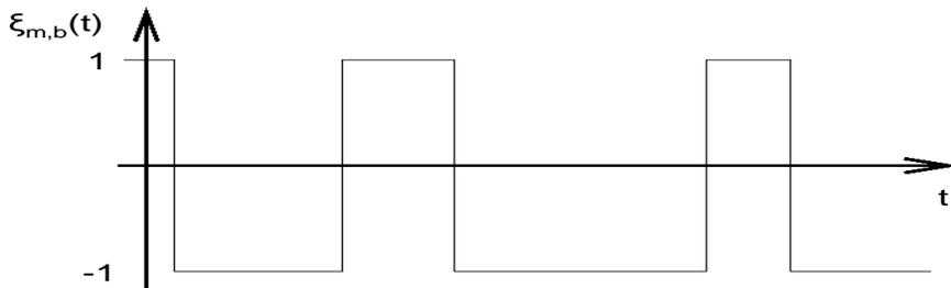
Fig.4 Normalized binary valued EEG signal  $\xi_{m,b}(t)$  with zero mean vs.  $t$
