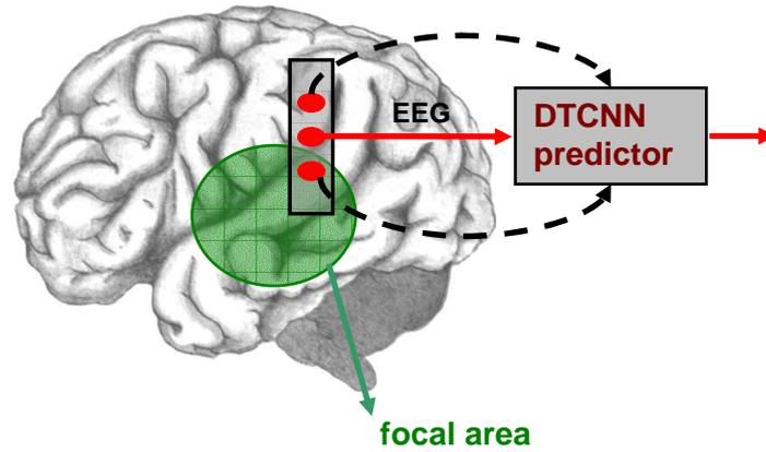
Fig. 2b Prediction scheme for EEG signals using single layer DTCNN whereas signal values (dashed line) of neighbouring electrodes will be considered in the signal prediction. AD conversion and pre-processing steps are not shown for the sake of convenience
