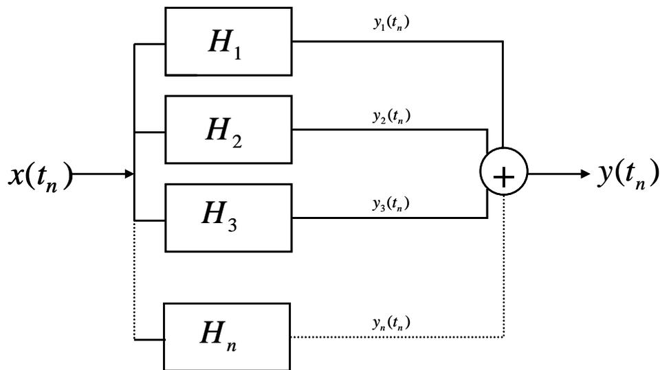
Fig. 1 n-th order Volterra system
