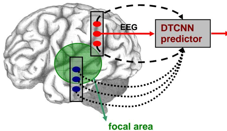
Fig. 2c Prediction scheme for EEG signals using multilayer DTCNN whereas signal values (dashed line) of neighbouring electrodes and of different electrode arrays (dotted line) will be considered in the signal prediction. AD conversion and pre-processing steps are not shown for the sake of convenience
