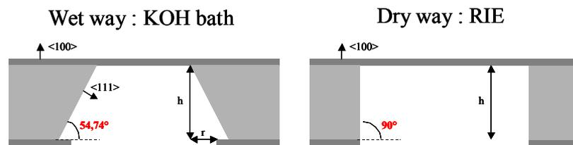
Figure 4. Schematics of the two silicon etching types : a) wet and b) dry
