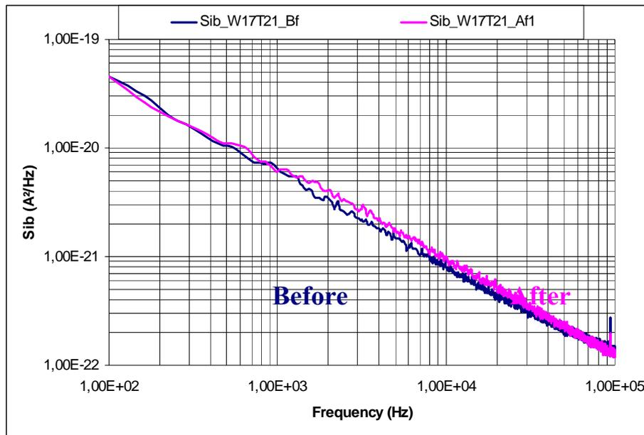
Figure 8. Low frequency noise spectrum density on the base current before and after BCB process
