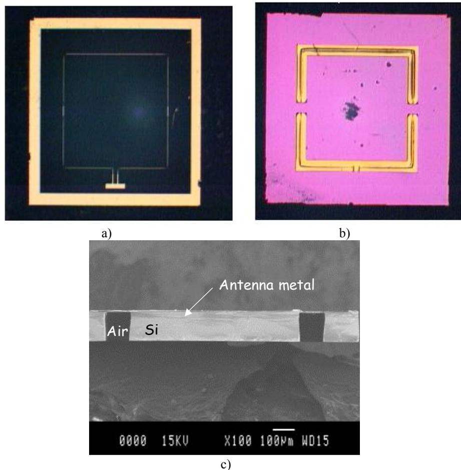
Figure 7. Pictures of an antenna with trenches seen from: a) the front side, b) the back side and c) the SEM cross section
