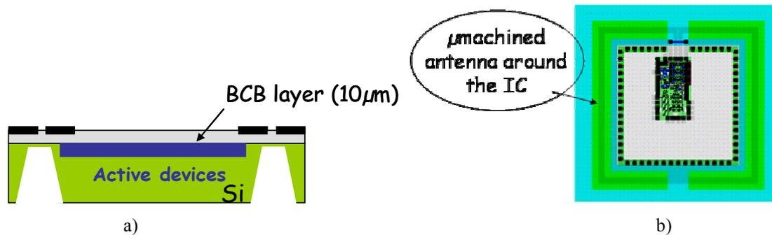
Figure 1. Schematics of an antenna with micromachined trenches: a) cross section and b) top view
