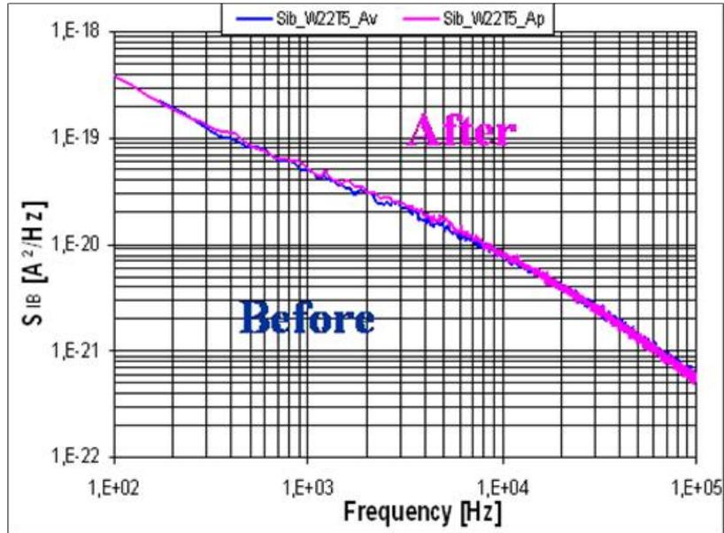
Figure 9. Low frequency noise spectrum density on the base current before and after BCB process
