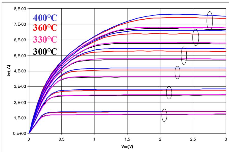
Figure 3. Static performances of a test transistor during a temperature ramp
