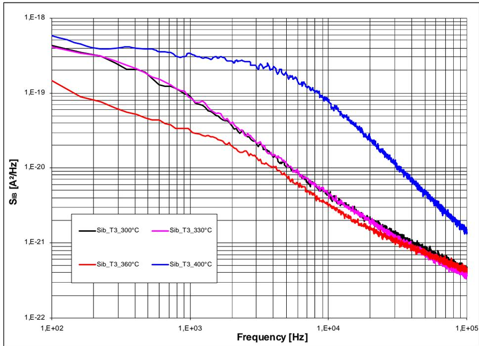
Figure 2. Low frequency noise spectrum density on the base current during a ramp temperature
