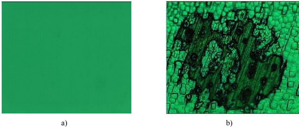
Figure 5. PECVD silicon nitride on a) standard silicon wafer and b) SiGe wafer
