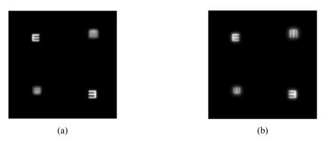
Figure 3. One of the elemental images captured with: (a) a conventional microlens array and (b) an amplitude-modulated microlens array. The 3D scene object contains tumbling charts located at different distances.
