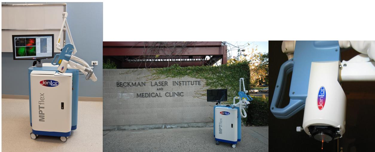
Fig. 1. Images of the Prism-Award winning device multiphoton tomograph MPTflex™. The scan head consists of a 3D scanning module, the focusing optics, two detectors for fluorescence and SHG imaging, and a 1.7 mm thick microendoscope. Photo (left) taken by Paul Kennedy.
