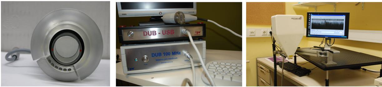
Fig. 5. The dermoscope Fotofinder, clinical ultrasound systems up to 100 MHz, and a 4beam-swept source OCT present state-of-the-art imaging tools in dermatology.
