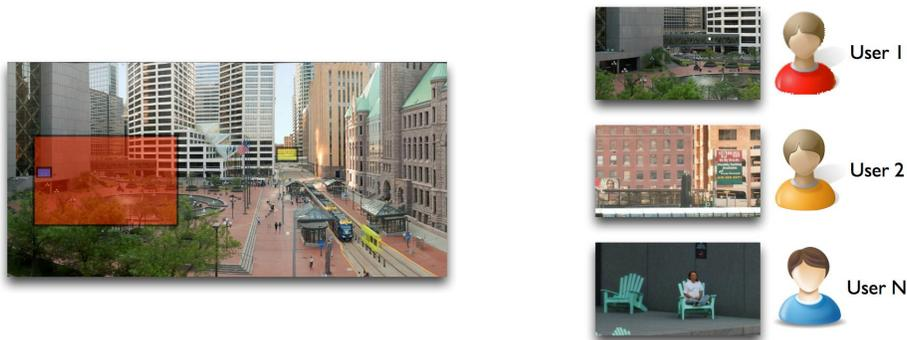
Figure 5. Multiple users can interact with the camera array simultaneously. Each user can have a window of any scale or position without interfering with other users. (Image courtesy of Tom Nelson [17]).
