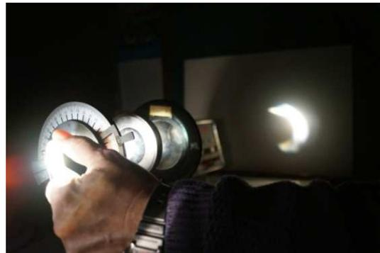
Figure 6. We place a plastic material between the two crossed polarizers and exert a pressure on the material, changing the chain of molecules. This turns the plastic into a birefringent material.
