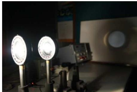
Figure 4. Two crossed polarizers result in a bluish screen since the efficiency of polarizers is not one hundred per cent and depends on the wavelength of the light. These polarizers are less efficient for the blue part of the spectrum.
