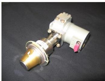
Figure 2: MARS MW IDDCA integrated in NOMAD instrument
