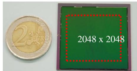
Figure 7 Sofradir test vehicle 2K<sup>2</sup> - comparison with 2 euros coin and size comparison between the test vehicle and the nominal size of 2048<sup>2</sup> detector
