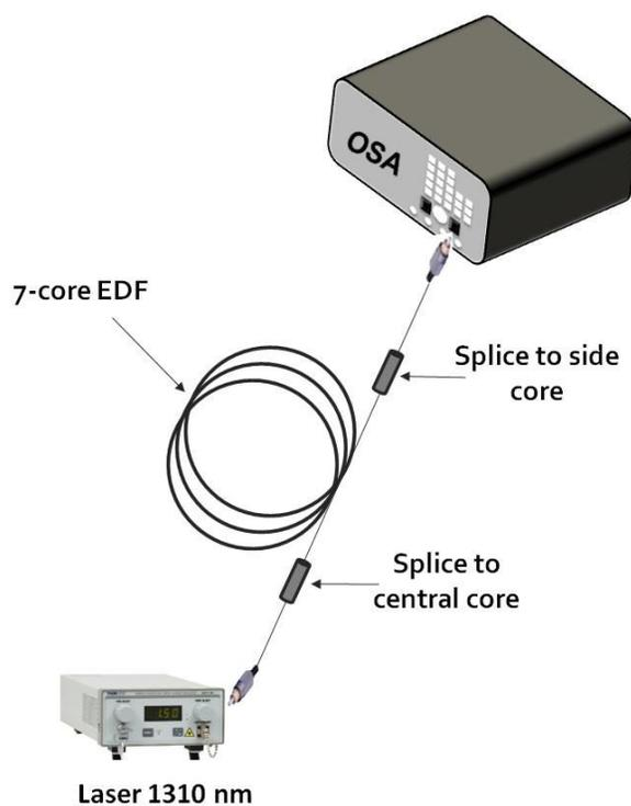
Fig. 4. Set-up for crosstalk evaluation.
