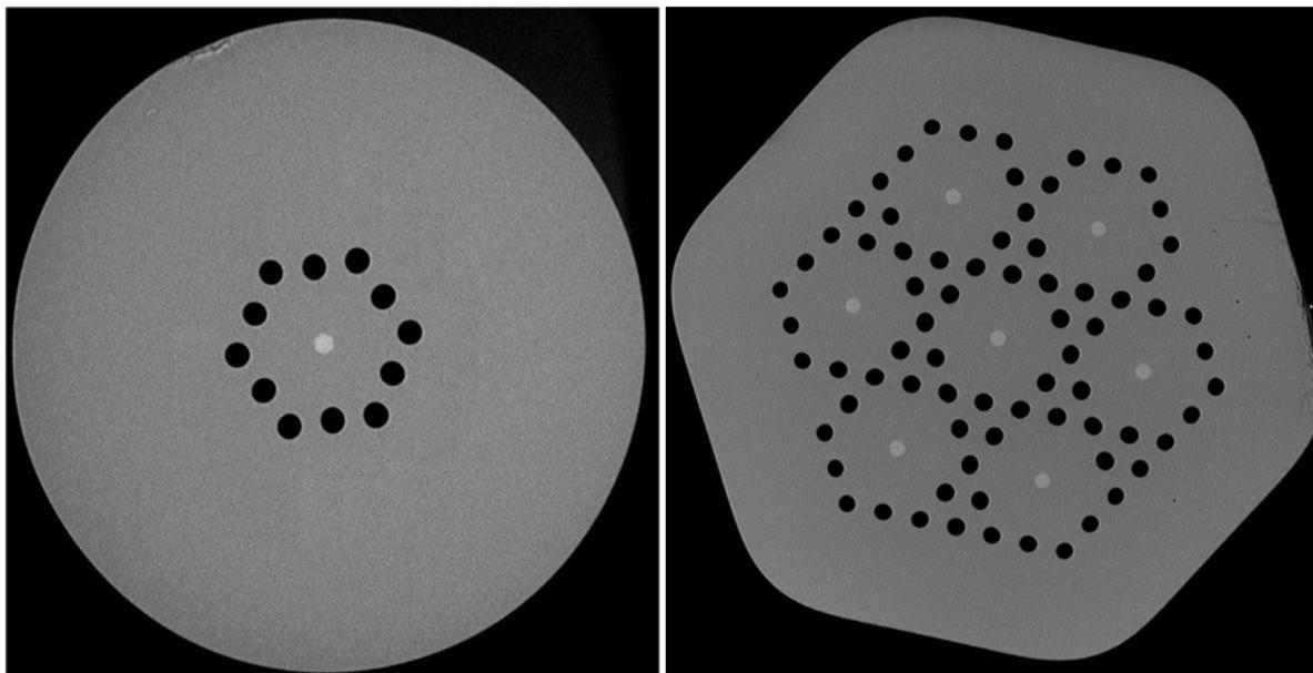
**Fig. 1.** SEM image of (left) elementary cell (single core EDF) and b) 7-core EDF.
