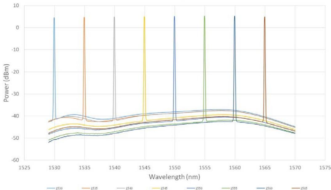
Fig. 7. Post-irradiation BEACON breadboard amplifier spectrum
