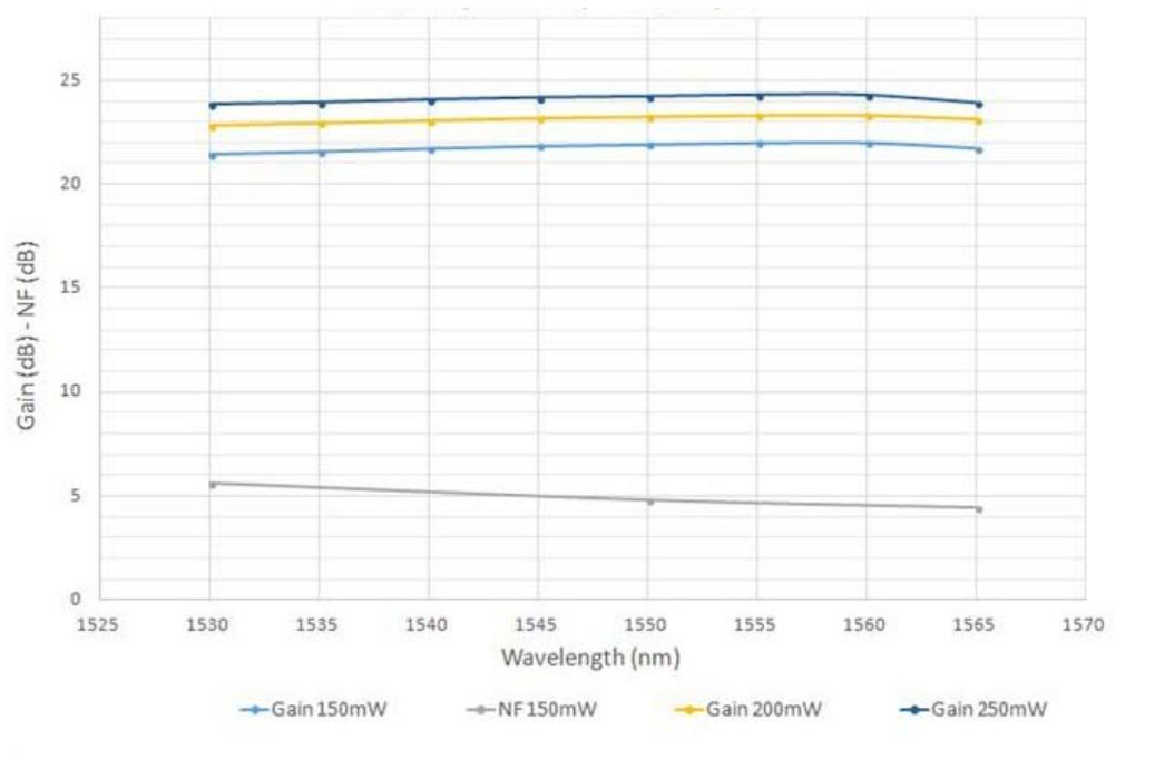
Fig. 6. Post-irradiation gain and NF performance of BEACON breadboard amplifier
