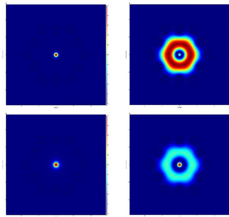
**Fig. 2.** Cross sections of modes propagating in the elementary cell of the seven core fibre. (top) Cross section for 980 nm and (bottom) Cross section for 1550 nm
