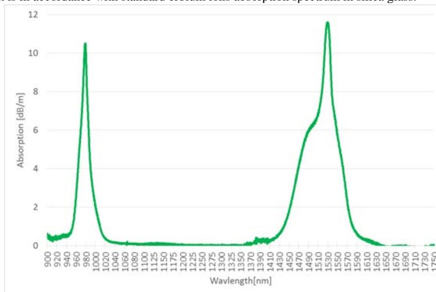
Fig. 3.: Absorption spectrum of manufactured EDF fiber.
