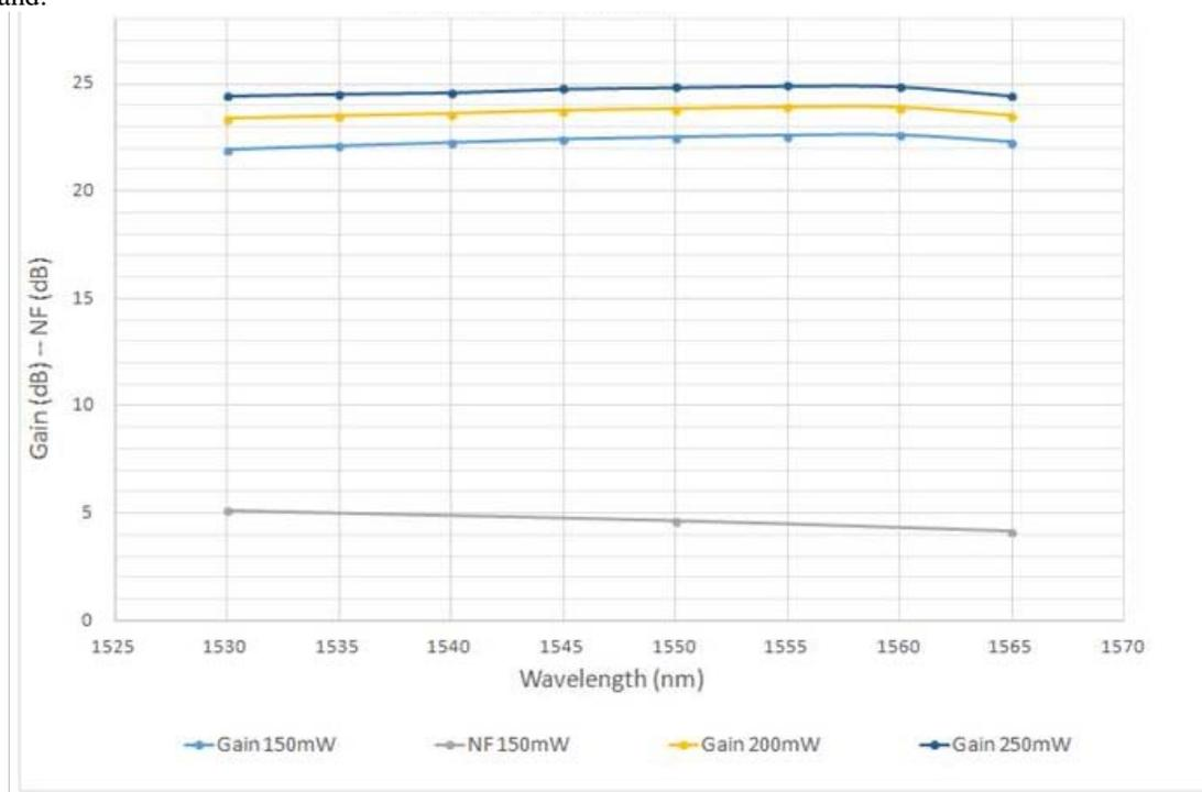
**Fig. 5.** Pre-irradiation gain and NF performance of BEACON breadboard amplifier
