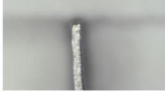
**Fig. 6.** Cross section of a 25  $\mu\text{m}$  thick aluminum foil, coated on both sides by Acktar black, magnification of x100
