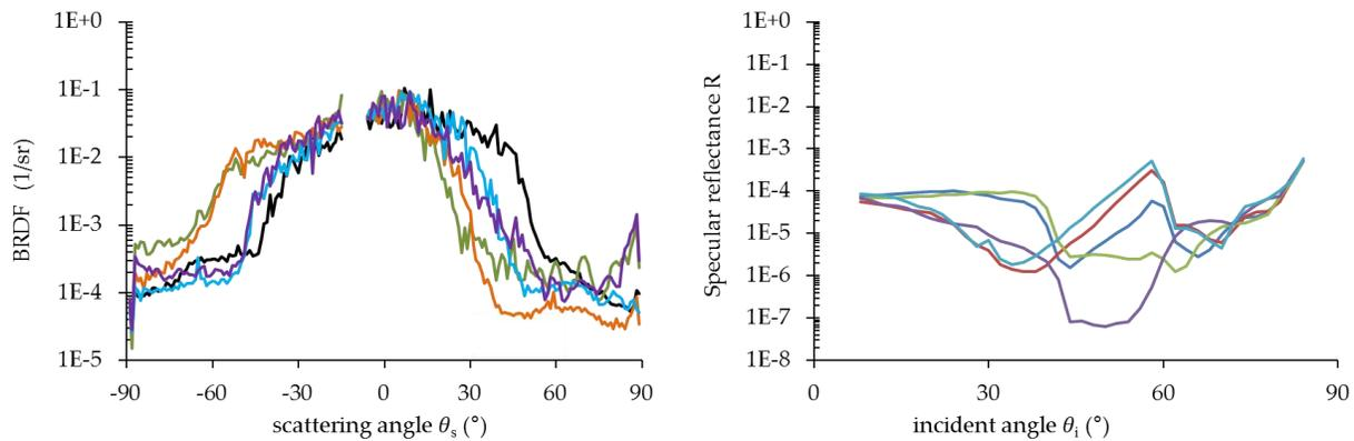
**Fig. 9.** BRDF (left,  $10^\circ$  angle of incidence) and reflectance (right) measurements performed at 5 different measurement positions, respectively
