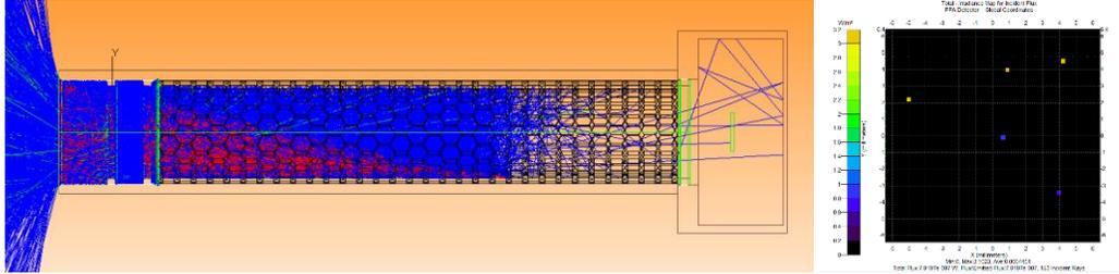
**Fig. 11.** Ray tracing simulation (left) - A lens doublet was placed in the left side of the tube, the detector was placed in the right side. Total irradiance map of the incident flux on the detector (right).
