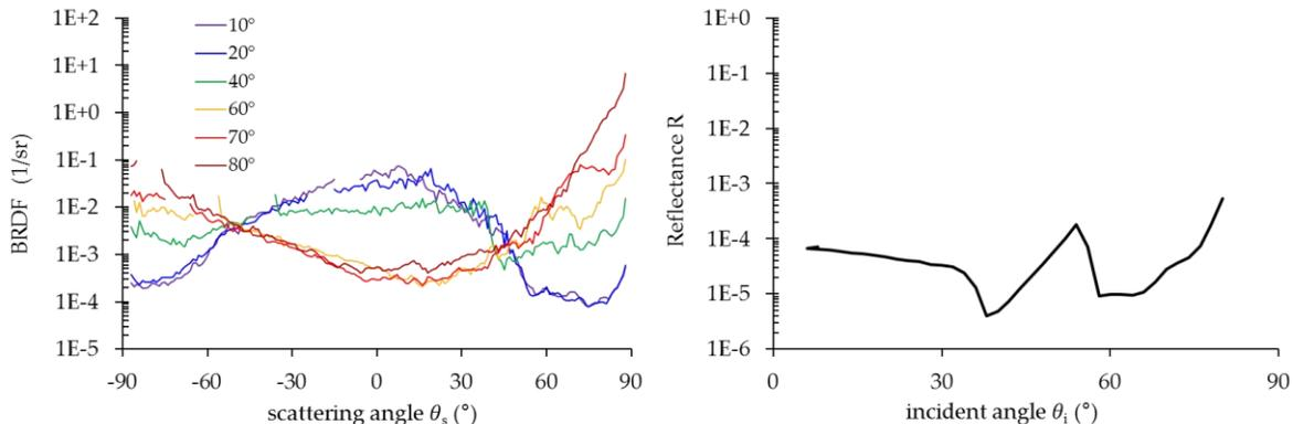
**Fig. 10.** BRDF (left) and reflectance (right) averaged from 5 different measurement positions, respectively
