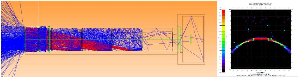
**Fig. 12.** Ray tracing simulation (left) - five vanes were placed in the tube to achieve the same FOV as in the first simulation. The detector was placed in the right side. Total irradiance map of the incident flux on the detector (right).
