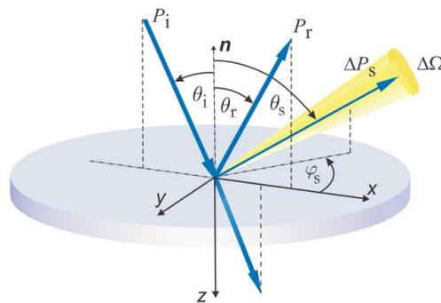
**Fig. 1.** Geometry for the definition of light scattering and specular quantities:  $\mathbf{n}$  sample normal;  $P_i$  – incident light power at the incidence angle  $\theta_i$ ;  $P_r$  – specularly reflected light power;  $\Delta P_s$  – scattered light power into detector solid angle  $\Delta\Omega$ .
