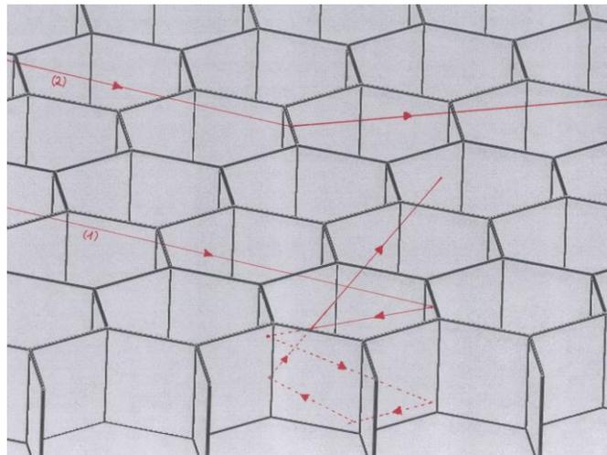
**Fig. 5.** Path of the stray light as reflected from the honeycomb structured surface. Path (1) will lose most of the power after 4 reflection from honeycomb wall (reflection from bottom plane not counted as not coated with Acktar Magic Black™). Path (2) will lose 0.01 of the power and reflected directly to the detector.
