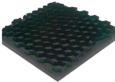
**Fig. 8.** The black surface on an aluminum substrate (for illustration contrast and brightness of the picture were enhanced)
