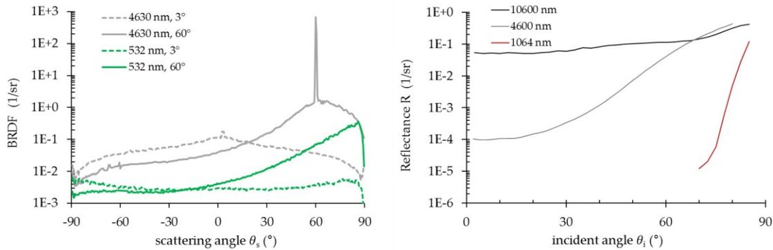
**Fig. 2.** Left: BRDF measurements at 532 nm and 4630 nm illumination wavelength on a black coating (Acktar Magic Black™ [3]) at different incident angles (3° and 60°). TS values were determined to 1% (532 nm, quasi normal incidence) and 15% (4630 nm, quasi normal incidence). Right: Measured specular reflectance (Acktar Magic Black™) as a function of the incident angle for different illumination wavelengths.
