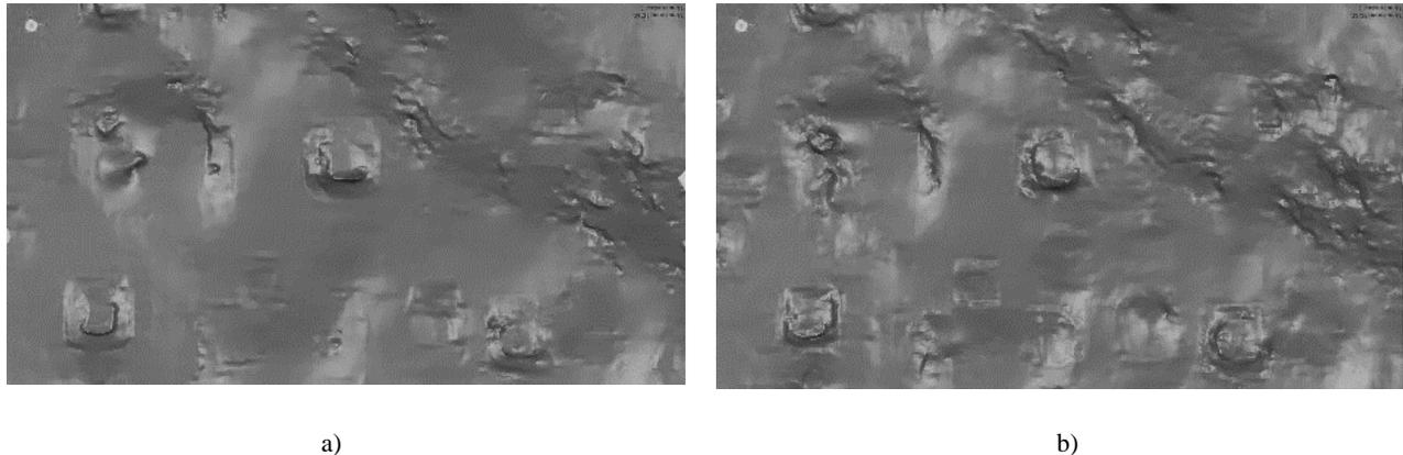
**Fig. 7** Level of detail of the DTMs processed in the example case of T25 by the using of (a) the Affine model approach and (b) the Polynomial model.
