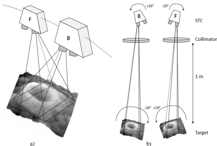
**Fig. 2** Setup for STC stereo validation concept: a. STC observing Mercury surface at periherm (flight conditions). b. In laboratory simulation of STC observing with “Forward channel” (F) and “Backward channel” (B) at periherm by means of the stereo validation setup.
