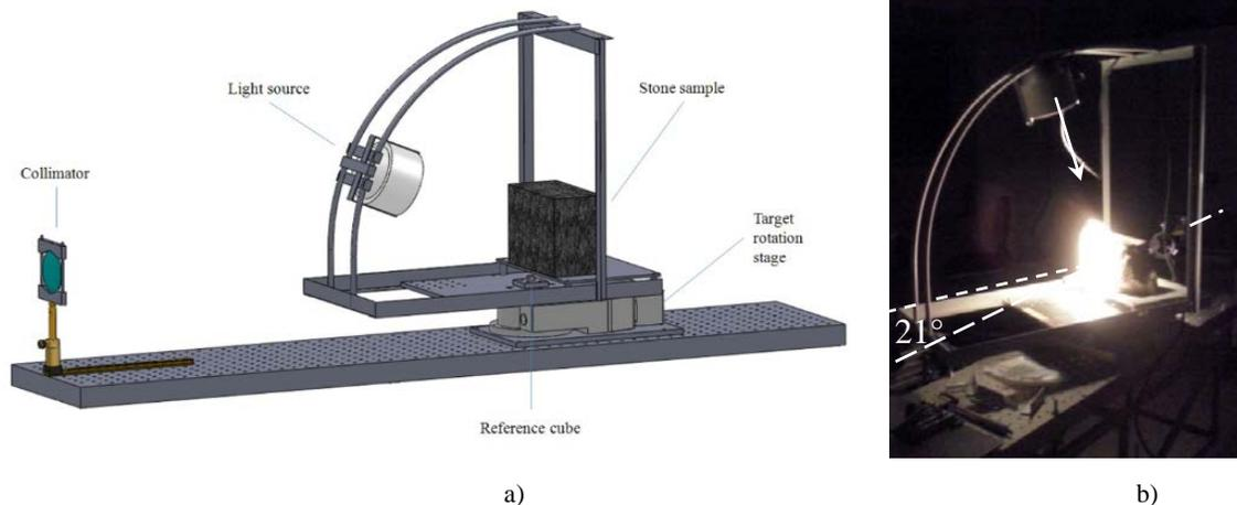
**Fig. 3** In (a) Setup for the stereo validation: mechanical layout. From left side: on the optical bench the collimator, on the rotation stage the light source and the rock sample. In (b) example of target (stone) acquisition with lamp in extreme orientation position and rotational stage on optical path of high channel in panchromatic ( $-21^\circ$ ).
