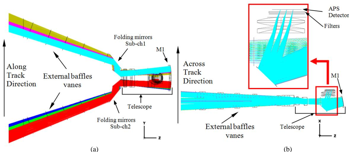
**Fig. 1** STC optical layout. In (a) the configuration is viewed in the plane defined by the along track and nadir directions; in (b) the projection in the orthogonal plane, the one including across track and nadir directions, is depicted. In the inset, an enlarged view of the focal plane region helps to better follow the rays optical path.
