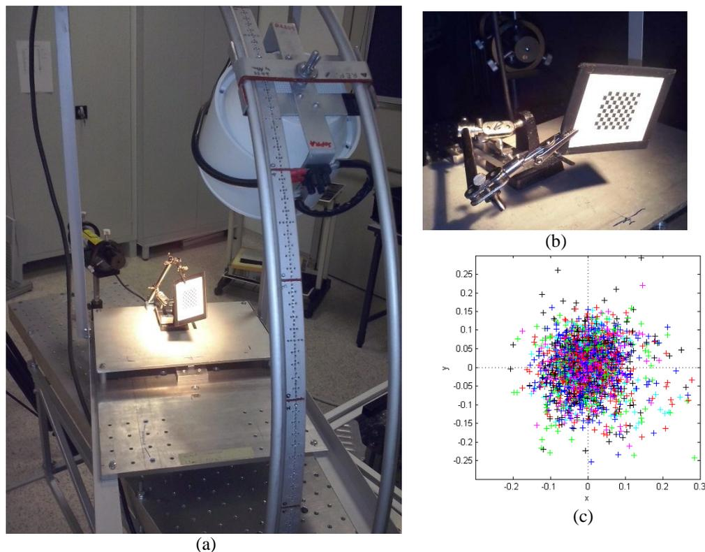
**Fig. 4** In (a) laboratory acquisition of the stereo target well lit by halogen lamp. In (b) the chessboard calibration target imaged with STC FM. In (c) the re-projection error from a calibration session. The 2- $\sigma$  curve of the error obtained in calibration is close to 0.1 pixel both along x and y directions.
