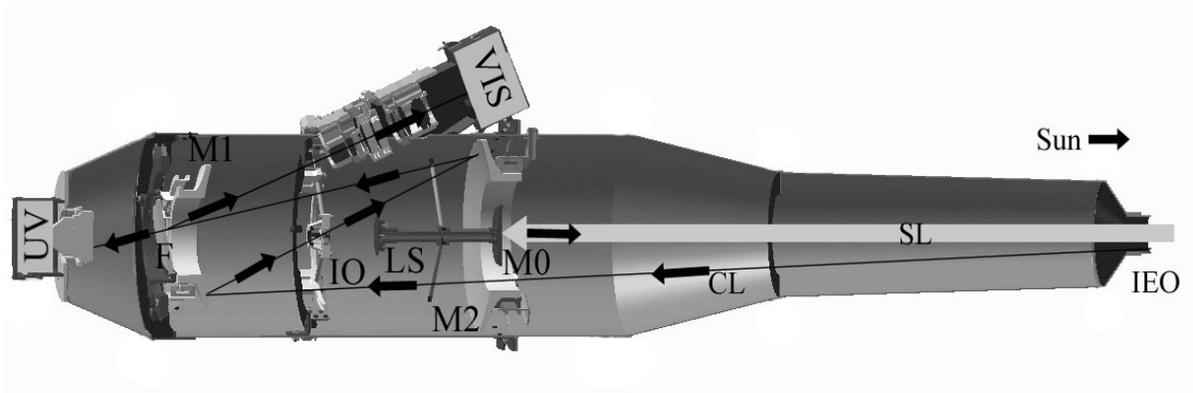
**Fig. 2.** Optomechanic structure of METIS. IEO is the Inverted external occulter, SL is the solar disk light incoming and rejected by the M0 rejection mirror, CL is the (coronal) light target. M1 and M2 constitute the on-axis gregorian telescope, UV and VIS are the detectors for the UV and visible channels, LS is a Lyot Stop and IO is the internal occulter. F is the Al+MgF<sub>2</sub> filter which splits the visible light and the HI line.
