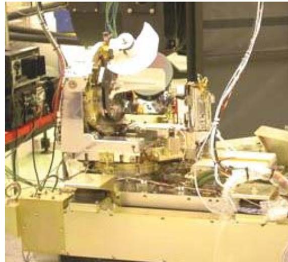
Fig.5: LOLA optical terminal during modal survey
