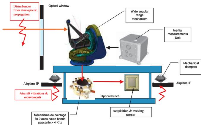
Fig.8: Pointing, Acquisition & tracking architecture
