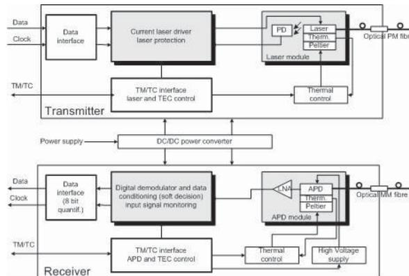
Fig.10: Laser communication unit
