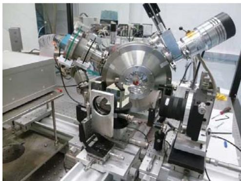
Figure 7. Cryogenic chamber installed on our interferometric setup. MMA with  $64 \times 32$  micromirrors is integrated ( $100 \times 200\ \mu\text{m}^2$  micromirrors).
