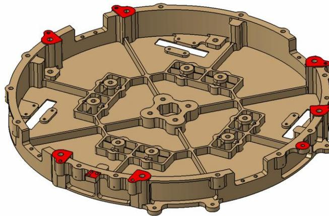
Figure 3: CCD Support Structure design
