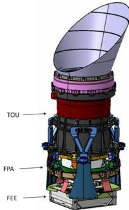
Figure 1: PLATO Camera 3D Model
