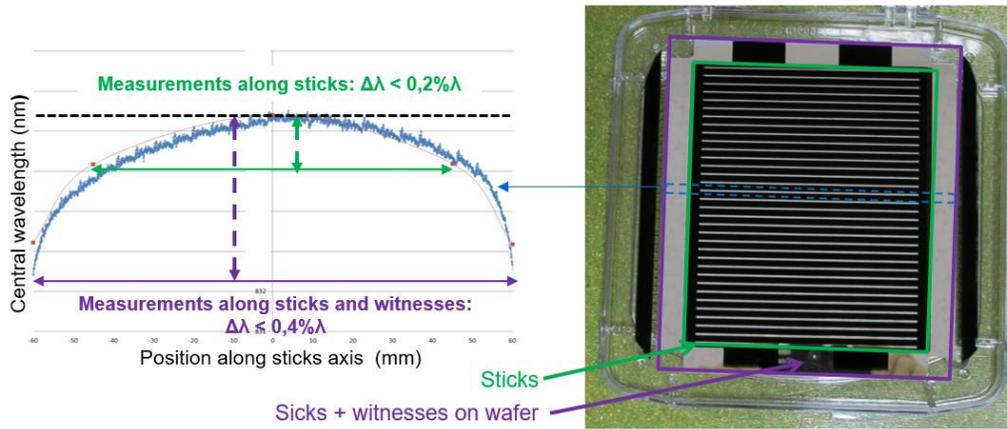
Fig. 7 shows the spectral uniformity along the sticks and witness areas on a black chrome masked wafer.
