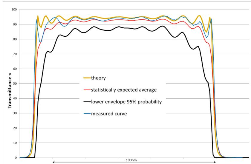
Fig. 5 shows the comparison of the measured curve of a magnetron sputtered filter (blue) with the theoretical design curve (yellow), the statistically expected mean curve (red) and lower envelope of the 95% probability corridor (black) of 500 simulated test runs.
