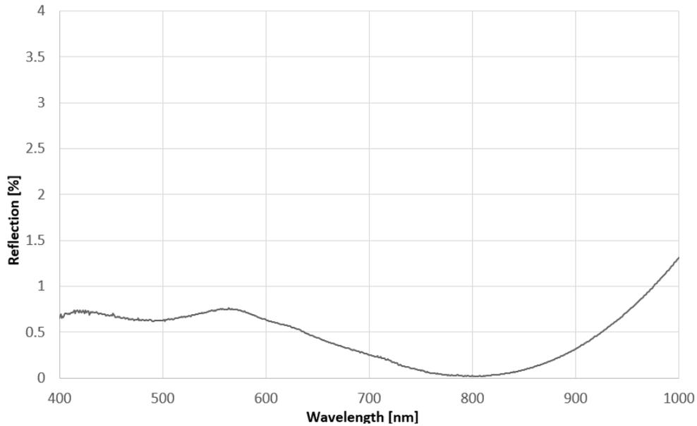
Figure 7: measured reflection spectrum of a black chrome coating adapted for the broadband filter discussed above.
