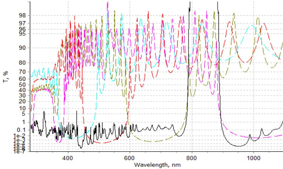
Fig. 2 Broadband filter design based on 4 differently centered quarterwave mirror stacks with about 100 layers. The individual mirror stacks are displayed in discontinued curves and different colors. The optimized final design is the black continuous curve.
