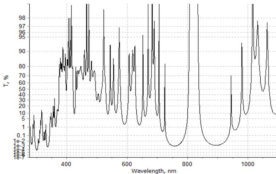
Fig. 1 Fabry-Perot filter design with 40 layers and 5 cavities and a FWHM of 35nm. To achieve a broad blocking one would have to add 60-80 layers.
