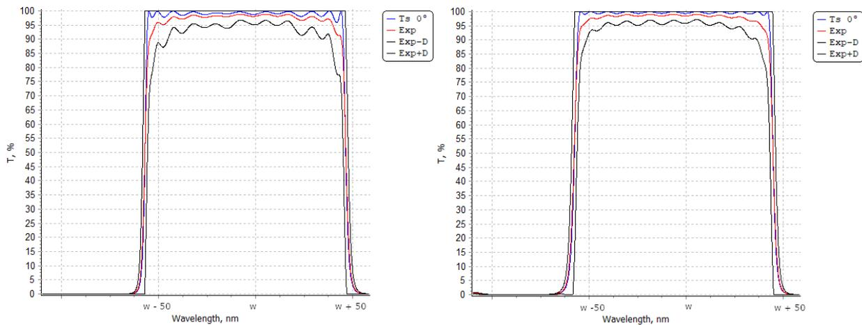
Fig. 3: error analysis for two candidate designs. The blue curve is the theoretical design, the red curve is the statistically expected mean curve, the lower and the upper black curves determine the tolerance channel for a preset probability corridor of 95%. Based on this fast test one would choose the design on the right hand side.
