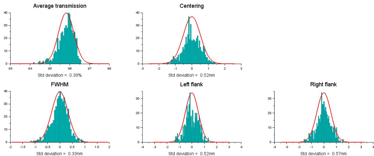
Figure 4 shows the results of the evaluation of the spectral characteristics of each of the 500 tests for average transmission, centering, FWHM, left flank and right flank. The Gaussian fits can then be evaluated for yield probability on a  $3\sigma$ -level for example.
