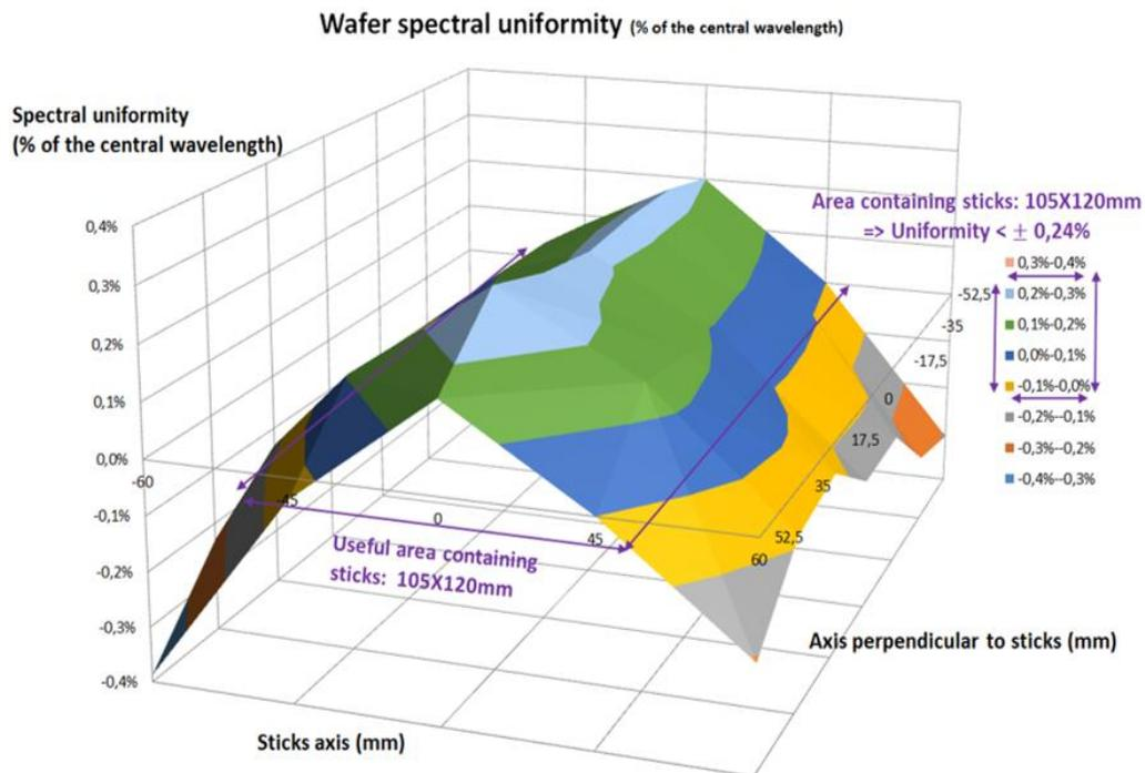
Fig. 6 shows the spectral uniformity of a magnetron sputtered filter in the useful area  $105 \times 120 \text{mm}$  of a non-masked wafer. The uniformity is below  $\pm 0.24\%$  over the surface where the sticks are located.
