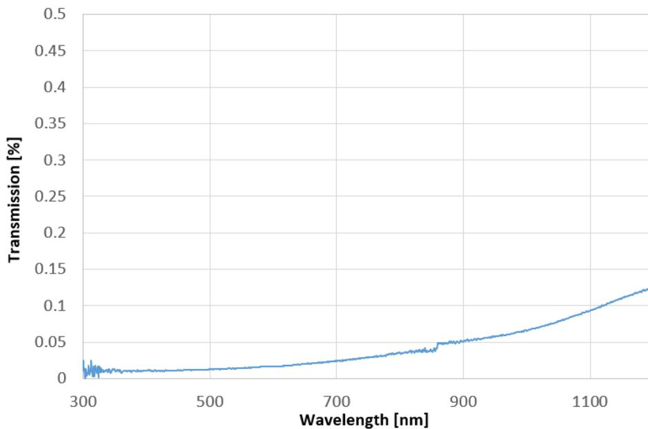
Figure 8: measured transmission spectrum of a black chrome coating adapted for the broadband filter discussed above.
