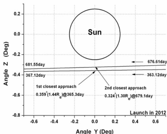
Fig. 4. Apparent angles during the two solar oppositions
