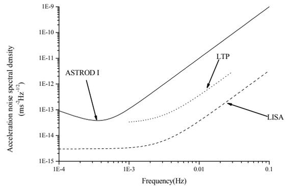
Fig.2. A comparison of the target acceleration noise curves of ASTROD I, the LTP and LISA.
