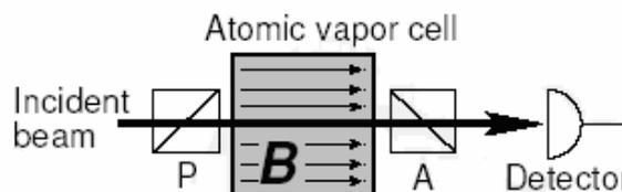
Fig. 5. FADOF work theory. P and A are crossed polarizing cube beam splitters (polarizer and analyzer)
