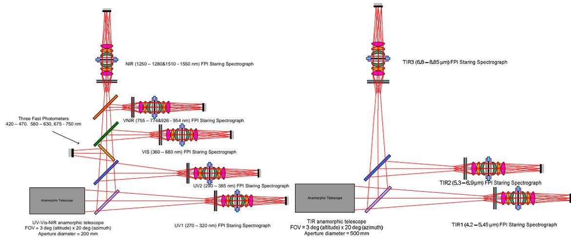
Fig. 3. Optical layouts of the SIMACC UV-VIS-NIR (left) and TIR (right) Spectrometer Modules.
