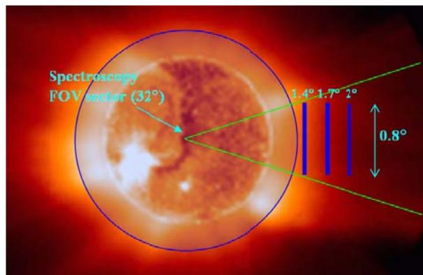
Fig. 6. Example at 0.28 AU of multi-slits FOV for the EUV spectroscopy path. The FOV sector for spectroscopy is about 32° out of the total 360° FOV. The remaining area is used for imaging.
