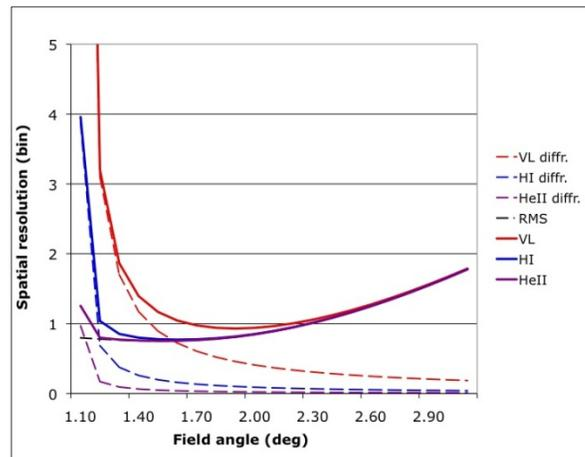
Fig. 5. Estimated METIS rms spatial resolution including diffraction as a function of the field angle. In this plot, continuous lines represent the total aberration, given by the quadratic sum of the rms spot diagram and the diffraction contribution (dashed lines). One bin corresponds to  $2 \times 2$  pixels ( $20 \times 20$  arcsec<sup>2</sup>).
