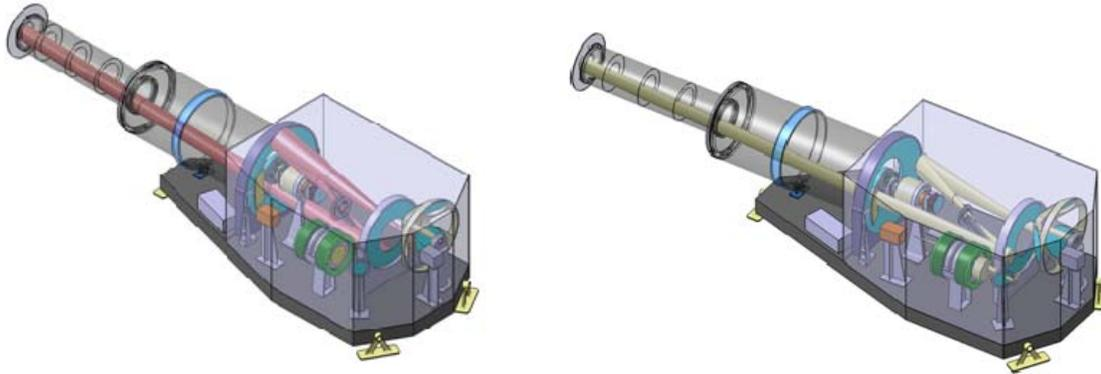
Fig. 3. Optical path inside METIS: ultraviolet (left), and visible (right).
