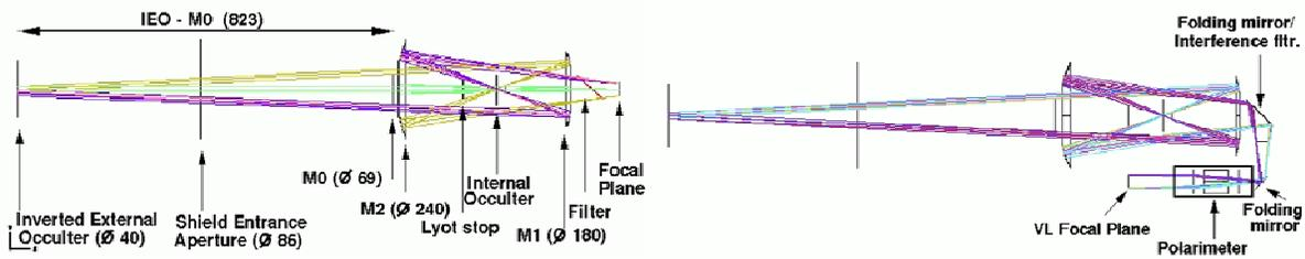
Fig. 4. METIS coronagraph optical ray tracing: ultraviolet path (left), visible path (right).
