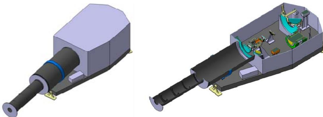
Fig. 1. Two different views of METIS layout. On the left, METIS is shown with its baffling system and enclosure: the thinned external cylinder is the baffling system protruding into the S/C heat shield and supporting the coronagraph external occulter. On the right, a cut-out of the instrument has been done to show the internal optical elements. In this figure, the main electronics box is not included.
