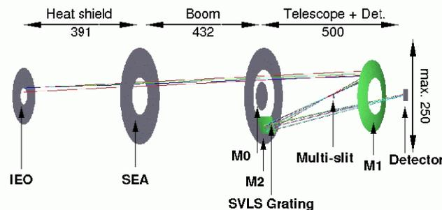
Fig. 7. Schematic layout of METIS spectroscopic channel. All the quotes are in mm.
