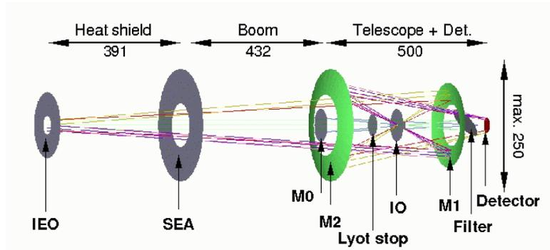
Fig. 2. Optical layout of the inverted coronagraph (only UV-EUV channel). Quotes are in mm. Acronyms are explained in the text.
