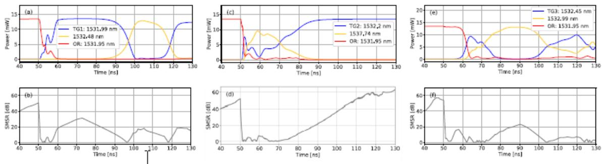
Figure 3 Simulation results for wavelength switching from 1531.95 nm for 3 different strategies: (a) and (b) switching to a neighboring longitudinal cavity mode 0.04 nm apart, (c) and (d) switching to the valley of the fine filter 0.25 nm apart, (e) and (f) switching to the neighboring peak of the fine filter 0.5 nm apart.
