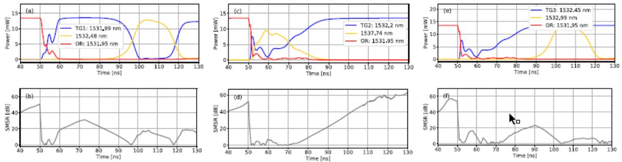
Figure 3 Simulation results for wavelength switching from 1531.95 nm for 3 different strategies: (a) and (b) switching to a neighboring longitudinal cavity mode 0.04 nm apart, (c) and (d) switching to the valley of the fine filter 0.25 nm apart, (e) and (f) switching to the neighboring peak of the fine filter 0.5 nm apart.
