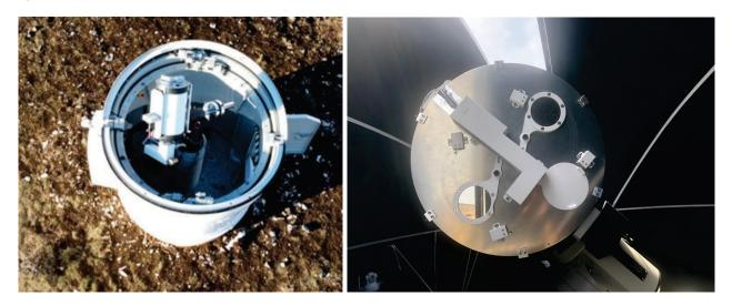
Figure 4. Left: the GMT instrument inside its 2.3m AllSky Baader dome. Right: The pupil mask and the optical device of the GMT instrument.
