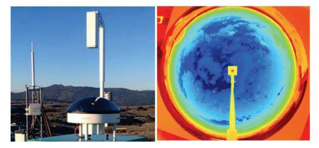
Figure 7. The Réuniwat Sky Insight IR camera installed on the roof of the MéO station at Calern Observatory (left). Right panel: example of sky image acquired by the Réuniwat Sky Insight IR camera.
