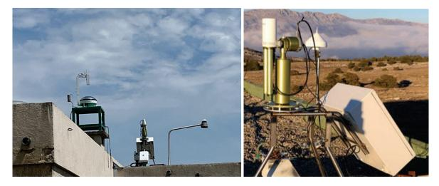
Figure 8. The Cimel CE318-T photometer installed near the Réuniwatt caméra on the roof of the MéO station at Calern Observatory.
