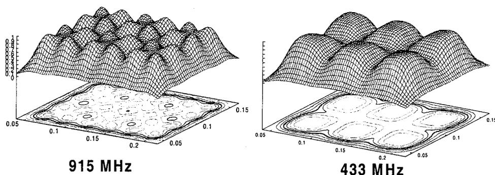
Fig. 5 - FDTD calculated SAR pattern 1 cm deep in muscle phantom under 6 element array of 4 cm square DCC apertures spaced 1.5 cm apart and coupled with 6.25 mm thick water bolus and driven at 915 or 433 MHz. Note that the bold contour, which represents 50% of SAR<sub>max</sub> in the 1 cm deep plane, extends to the array perimeter demarcated by the dashed aperture outlines.
