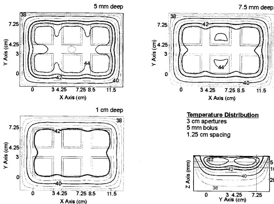
Fig. 6 - Temperature distribution predicted 5, 7.5 and 10 mm deep in muscle and central y-z cross section under 6 element array of 3 cm square DCC apertures coupled with 5 mm water bolus. Blood perfusion is assumed to be 2 kg/m<sup>3</sup>s, water bolus temperature is 42°C and highest temperature point in tissue is 45°C. Note the 42°C contour in bold extends to the array perimeter down to 1 cm depth in muscle.
