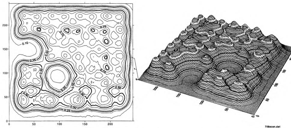
Fig. 4 - Measured relative SAR distribution 1 cm deep in muscle phantom from a 16 element array of 4 cm square DCC apertures spaced 1.5 cm apart, radiating through a 12 mm thick water bolus. Two apertures are off to demonstrate the resolution of power control of the antenna array. The two bold lines are 25% and 50% of  $SAR_{max}$ .
