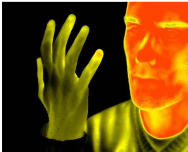
Figure 2. An image taken with a superlattice FPA at MP Technologies with the following parameters: detector array size  $320 \times 256$ , pixel pitch  $30 \mu\text{m}$ , cutoff wavelength  $11 \mu\text{m}$ , operating temperature 81 K, integration time 0.11 ms, average detectivity about  $10^{11}$  Jones, and operability 96%.
