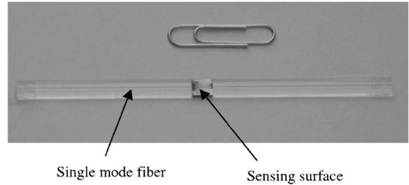
**Fig. 3** Photograph of the D-type optical fiber sensor.
