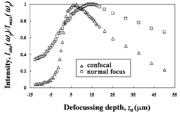
**Fig. 4** Normalized plot of probe response functions (*i.e.*, Raman band intensity  $I_{obs}(\omega_p)/I_{max}(\omega_p)$  for UHMWPE as a function of defocusing depth  $z_0$ ) for normal and confocal probe configurations.
