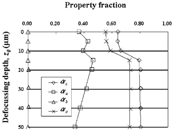
Fig. 13 *In-depth* profiles of crystalline, amorphous, orthorhombic, and third phases in the long-term retrieved acetabular cup. Probe resolution in this assessment was in the range  $z_d \approx 6.4 \div 10 \mu\text{m}$ .
