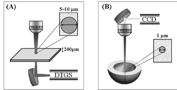
**Fig. 18** Schematic drafts for (A) FTIR (destructive) and (B) confocal Raman (nondestructive) assessments of oxidation index in UHMWPE. The required sample thickness for FTIR assessment and lateral spatial resolutions are explicitly shown. DTGS and CCD abbreviations stand for deuterated triglycine sulfate and charge-coupled device, respectively.
