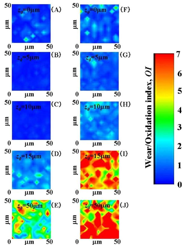
Fig. 10 Maps of wear index (related to oxidation index) collected at increasing depths of focal plane  $z_0$  of the confocal probe on the long-term retrieved UHMWPE acetabular cup shown in Fig. 1(C): (A) through (E) refer to the nonwear zone, while (F) through (J) refer to the main wear zone of the retrieved cup.
