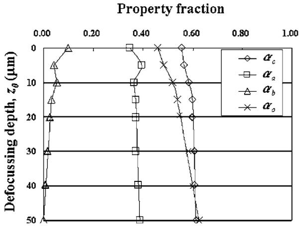
Fig. 12 *In-depth* profiles of crystalline, amorphous, orthorhombic, and third phases in the short-term retrieved acetabular cup. Probe resolution in this assessment was in the range  $z_d \approx 6.4 \div 10 \mu\text{m}$ .
