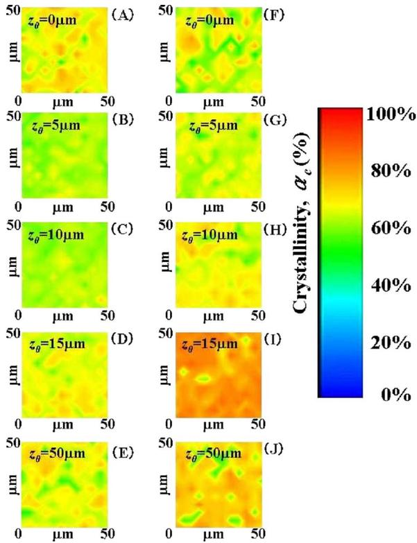
Fig. 7 Maps of crystalline phase volume fractions collected at increasing depths of focal plane  $z_0$  of the confocal probe on the long-term retrieved UHMWPE acetabular cup shown in Fig. 1(C): (A) through (E) refer to the nonwear zone, while (F) through (J) refer to the main wear zone of the retrieved cup.
