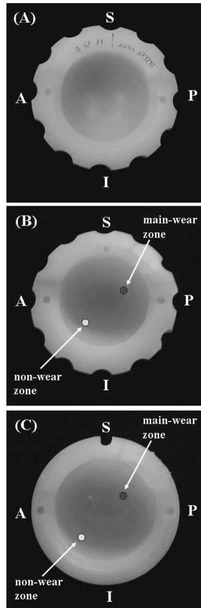
**Fig. 1** Photographs of the investigated hip acetabular cups: (A) new cup; (B) short-term retrieved cup; and (C) long-term retrieved cup. The surface of each cup was irradiated by a  $\gamma$ -ray dose of 33 kGy.
