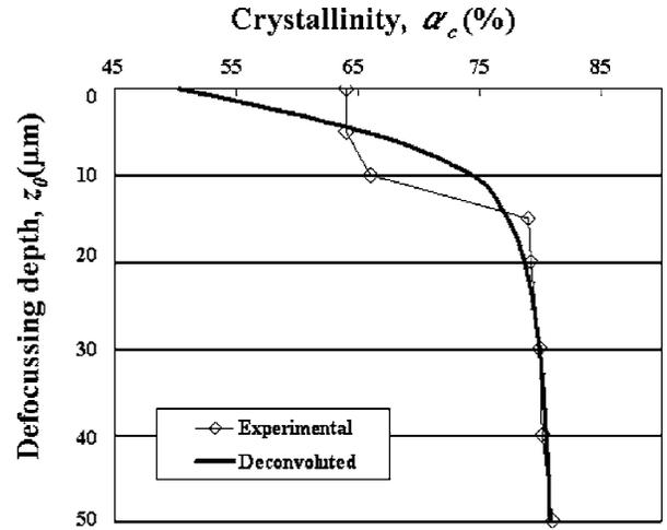
Fig. 15 Plots of crystallinity phase fraction distribution along the *in-depth*  $z$  axis as experimentally detected by the confocal probe and after mathematical probe deconvolution according to Eq. (20). In the calculation, Eq. (21) was adopted as the trial function, and best fitting was obtained with  $a$ ,  $b$ ,  $c$ , and  $d$  equal to 0.60, 0.14, 0.25, and  $-0.83$ , respectively.
