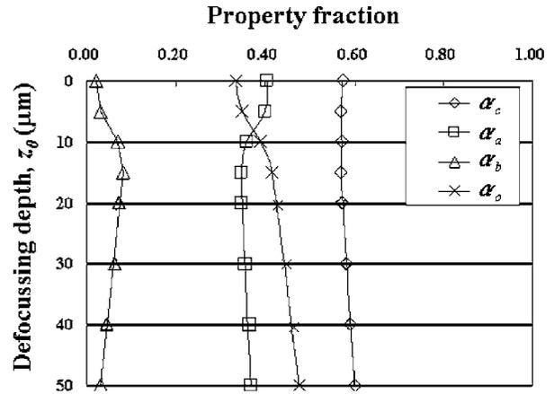
Fig. 11 *In-depth* profiles of crystalline, amorphous, orthorhombic, and third phases in the new acetabular cup. Probe resolution in this assessment was in the range  $z_d \approx 6.4 \div 10 \mu\text{m}$ .
