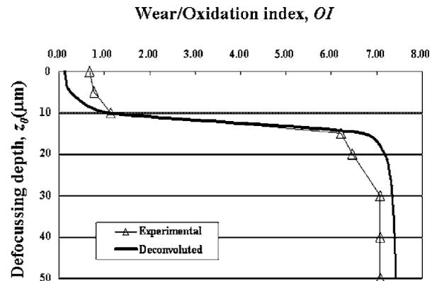
Fig. 16 Plots of wear index (related to oxidation index) distribution along the *in-depth*  $z$  axis as experimentally detected by the confocal probe and after mathematical probe deconvolution according to Eq. (20). In the calculation, Eq. (21) was adopted as the trial function, and best fitting was obtained with  $a$ ,  $b$ ,  $c$ , and  $d$  equal to 3.7, 2.4, 1.0, and  $-12.0$ , respectively.
