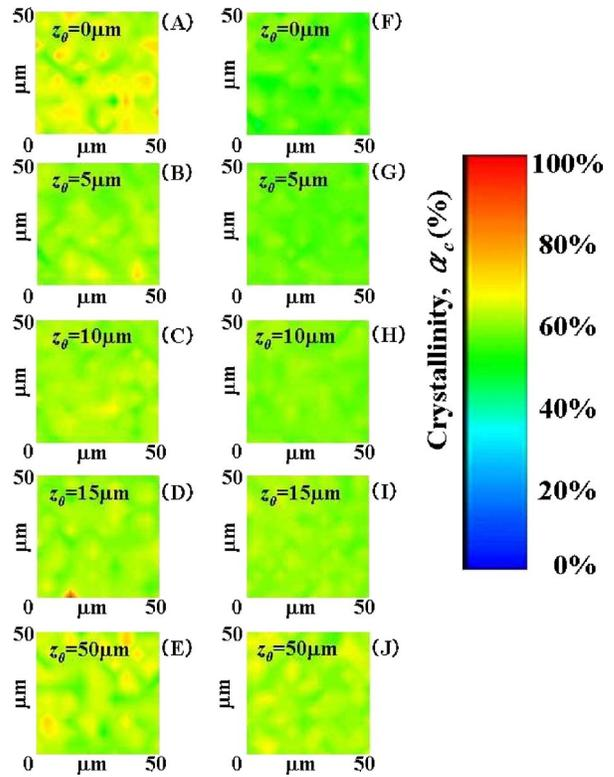
Fig. 6 Maps of crystalline phase volume fractions collected at increasing depths of focal plane  $z_0$  of the confocal probe on the short-term retrieved UHMWPE acetabular cup shown in Fig. 1(B): (A) through (E) refer to the nonwear zone, while (F) through (J) refer to the main wear zone of the retrieved cup.
