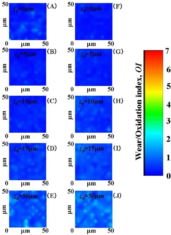
Fig. 9 Maps of wear index (related to oxidation index) collected at increasing depths of focal plane  $z_0$  of the confocal probe on the short-term retrieved UHMWPE acetabular cup shown in Fig. 1(B): (A) through (E) refer to the nonwear zone, while (F) through (J) refer to the main wear zone of the retrieved cup.
