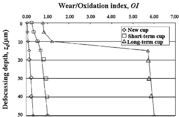
Fig. 14 *In-depth* profiles of wear/oxidation index in new, short-term, and long-term retrieved acetabular cups. Probe resolution in this assessment was in the range  $z_d \approx 6.4 \div 10 \mu\text{m}$ .
