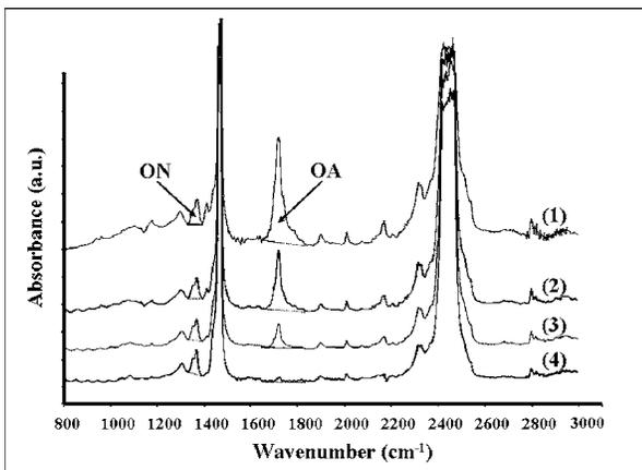
**Fig. 20** IR spectra collected on a virgin UHMWPE cup after “controlled” experiments in an oxidizing atmosphere. These spectra correspond to the data points indicated by arrows in Fig. 19.  $OI$  was calculated according to ASTM standard<sup>28</sup> from the areas below the absorption curve as  $OI=OA/ON$ . The baseline curves are also explicitly indicated by broken lines.
