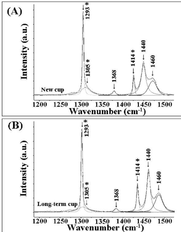
**Fig. 17** Portions of Raman spectra investigated to calculate the oxidation index according to Eq. (6): (A) average spectrum collected on a new acetabular cup; and (B) average spectrum collected on the long-term exposed *in-vivo* acetabular cup. Spectral fitting by Gaussian/Lorentzian subbands is shown for both spectra and the salient bands used for assessing *OI* located with an asterisk.
