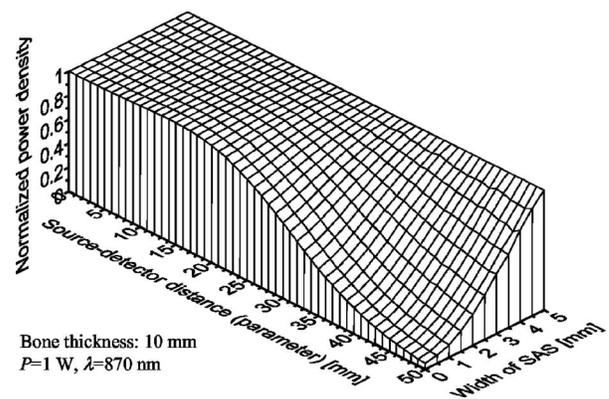
Fig. 3 Relative changes in received power density of NIR-BSR versus the width of the SAS for a given source-detector distance for head with scalp intact.
