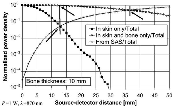
**Fig. 8** Relative contribution of radiation: transmitted in the skin only, transmitted in the skin and skull bone only, and propagated within the SAS, for head with scalp intact, in the total balance of NIR-BSR.
