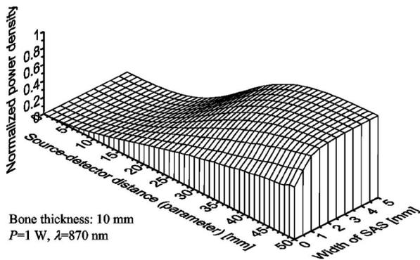
**Fig. 12** Contribution of radiation propagated within the SAS to the total NIR-BSR received by the detector as a function of source-detector distance and SAS width for the scalp-void part of the head.
