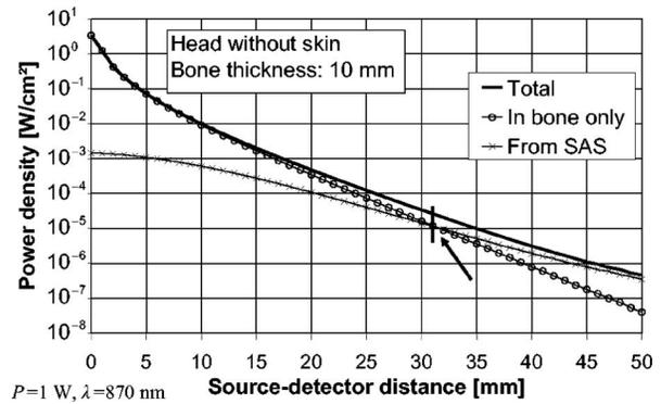
**Fig. 13** Power density of NIR-BSR on the surface of the head and the contribution of radiation: (a) transmitted within the skull bone only, and (b) propagated within the SAS, for SAS width 1 mm and source power of 1 W, for the scalp-void part of the head.
