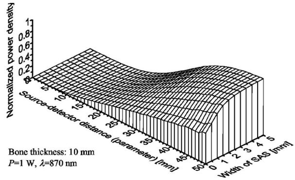
Fig. 6 Contribution of radiation propagated within the SAS to the total NIR-BSR received by the detector as a function of source-detector distance and SAS width for head tissues with scalp included.
