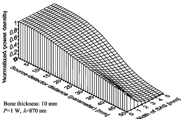
Fig. 5 Contribution of radiation propagated within the skin and bone only to the total NIR-BSR received by the detector as a function of source-detector distance and SAS width for the part of the head with scalp intact.
