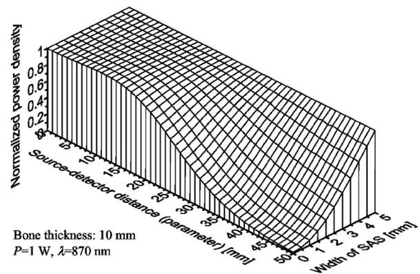
**Fig. 10** Relative changes in received power density of NIR-BSR versus the width of the SAS for a given source-detector distance for the scalp-void part of the head.
