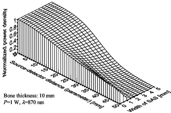
**Fig. 11** Contribution of radiation propagated within the skull bone only to the total NIR-BSR received by the detector as a function of source-detector distance and SAS width for the scalp-void part of the head.
