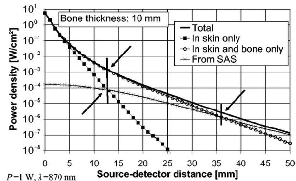
Fig. 7 Power density of NIR-BSR on the surface of the head and the contribution of radiation: transmitted within the skin only, transmitted in the skin and skull bone only, and propagated within the SAS, for SAS width 1 mm and source power of 1 W, for tissues of the head including the scalp.
