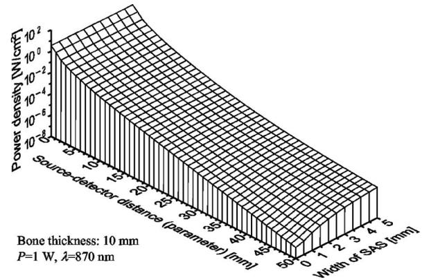
**Fig. 9** NIR-BSR power density on the surface of the scalp-void head as a function of source-detector distance and SAS width, for source power 1 W.
