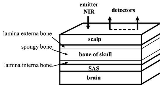
Fig. 1 Simplified diagram presentation of a vertical section of a block of tissues of the head, with NIR conducting layers identified.
