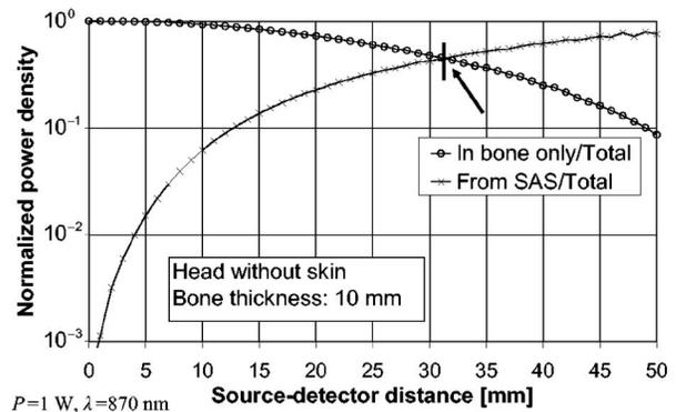
**Fig. 14** Relative contribution of radiation: (a) transmitted in the skull bone only, and (b) propagated within the SAS for the scalp-void part of the head, in the total balance of NIR-BSR.
