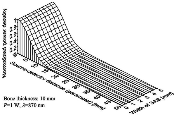
Fig. 4 Contribution of radiation propagated within the skin only to the total NIR-BSR received by the detector as a function of the source-detector distance and SAS width for part of the head with scalp intact.
