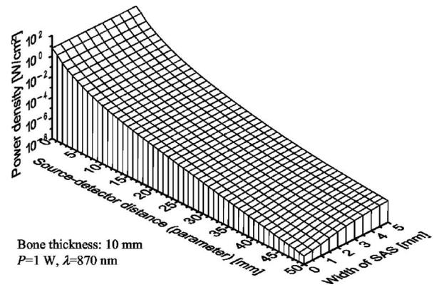
Fig. 2 NIR-BSR power density on the surface of the head with scalp intact as a function of source-detector distance and SAS width, for source power 1 W.
