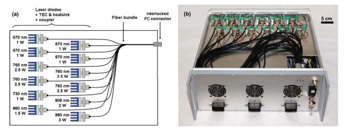
Fig. 2 Laser diode-based NIR light source: (a) Schematics of the NIR light source. Note the wavelength modules composed of one laser diode, a TEC with its heatsink, and an FC coupler. The wavelength modules are combined through a 12-to-1 fiber bundle. (b) Picture of the actual NIR laser light source with the top cover removed. Note the wavelength modules and the fiber bundle.
