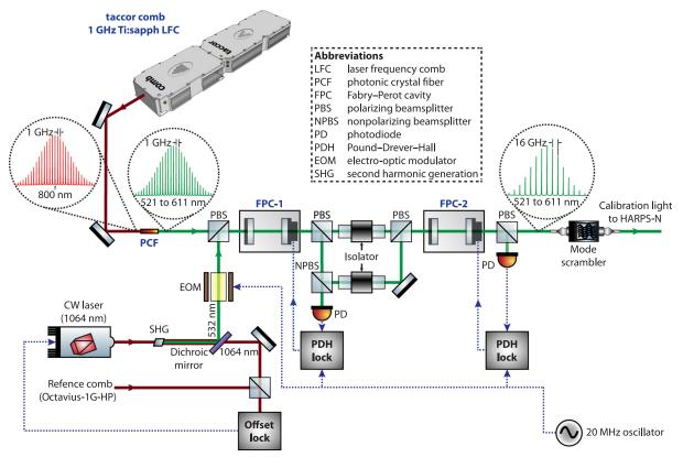
**Fig. 1** Astro-comb block diagram showing a turn-key LFC that generates 1-GHz-spaced comb teeth about a center wavelength of 800 nm, a commercial PCF that coherently shifts the light into the visible wavelength range, and custom-built FP cavities that suppress 15 out of every 16 lines to match the resolution of the astrophysical spectrograph to be calibrated. (Abbreviations defined in figure; see text for more details.)
