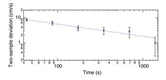
Fig. 3 Two-sample deviation of the measured frequency stability (in RV units) of the astro-comb versus averaging time. The black circles are the measured stability, and the dashed line is a fit consistent with the shot noise floor. The overall duration of the measurements was  $\sim$ 1 h.
