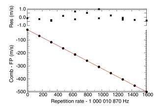
**Fig. 5** Measured mean difference in astro-comb spectral lines relative to a white-light FP spectrum (black circles) as a function of comb repetition rate, with a linear fit (red line) and residuals (top trace). The error bars of the residuals plot are the statistical uncertainty of  $\approx$ 10 cm/s (see text).
