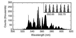
Fig. 2 Astro-comb spectrum measured with HARPS-N spectrograph. The strong peak at 532 nm is the CW reference laser used to stabilize the filter cavity lengths. Inset: at higher spectral resolutions, individual comb teeth (spectral lines) are observed.
