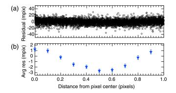
**Fig. 6** (a) Difference between expected and actual astro-comb peak position, as a function of peak position inside a pixel. The uncertainty for each point is consistent with the  $\sim$ 10 millipixel scatter observed. (b) Data shown in panel (a) averaged into bins with 0.1 pixel width.
