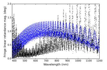
**Fig. 12** The amplitude of the linear retardance fringes in narrow spectral bandpasses of R = 10,000 spectral sampling for the SPINOR 3/8-wave modulator. Black is the linear retardance fringe magnitude using a 20- $\mu$ m air gap and a single-layer antireflection coating. Blue shows an uncoated model with crystals optically contacted. See text for details.
