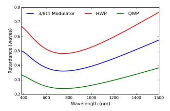
**Fig. 9** The linear retardance predicted for the three SPINOR bicrystalline achromats. SPINOR retarder designs at 633 nm wavelength are to 1/4-wave, 3/8-wave, and 1/2-wave retardance. The 1/4 wave is shown in green with crystals at (0.960209 and 1.098837 mm) thickness. The 3/8-wave retarder is shown in blue with crystals of (1.438883 and 1.648256 mm) thickness. The 1/2-wave retarder is shown in red with crystals at (1.920417 and 2.197675 mm) thickness.
