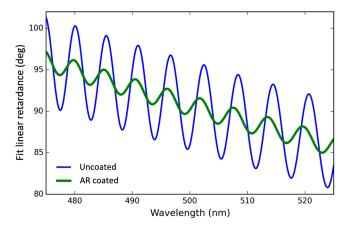
**Fig. 6** The linear retardance fit to a zero-order quartz crystal retarder of 13.587  $\mu$ m physical thickness. Blue shows uncoated. Green shows antireflection coated. The blue curve can be compared with Clarke.<sup>49</sup> We use the Sueoka<sup>10</sup> revised birefringence measurements, and we get a slightly different retardance than when using the CVI refractive indices giving 13.587  $\mu$ m as the exact zero-order retardance thickness for 500-nm wavelength.
