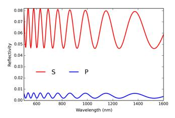
Fig. 2 The reflectivity for the thick isotropic  $MgF_2$  coating on a fused silica window at a 45-deg incidence angle. The reflectivity curves oscillate about their average values of 6.43% for *S*- and 0.43% for *P*-.
