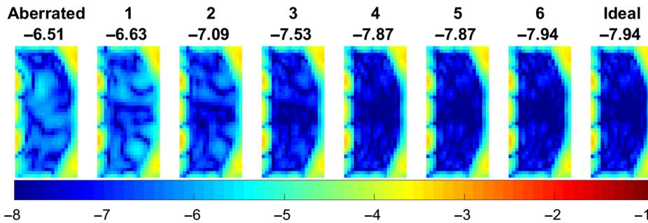
**Fig. 13** Evolution of the DF over the six iterations [seen in Fig. 14(b)] to converge from a degraded DF average contrast of  $10^{-6.51}$  to the LDFC-corrected DF with  $10^{-7.94}$  average contrast. The ideal DF is shown in the final frame for reference. Scale is  $\log_{10}$  contrast.
