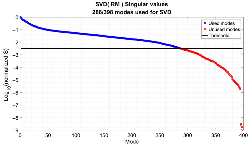
**Fig. 5** Singular values of the spatial LDFC response matrix  $M$  showing the applied SVD threshold (black) as well as the modes that were used in the inversion (blue) and the modes that were discarded (red). Out of 398 total modes, 286 were used for the inversion of  $M$  in the following simulations.
