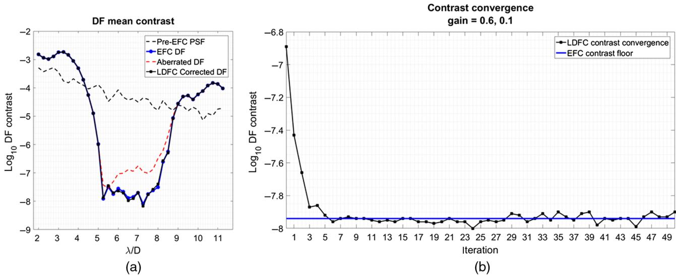
**Fig. 10** Performance of the spatial LDFC servo with a sinusoidal phase perturbation. Gain = 0.6 until the DF contrast reached  $10^{-7.9}$ . The gain was lowered to 0.1 for the remaining iterations. (a) Average contrast across the full DF for the pre-EFC PSF, DF post-EFC (blue), DF post-EFC with injected speckle (red), and the corrected DF post-LDFC (black). (b) Average DF contrast (black) over 50 iterations showing convergence to the initial EFC contrast (blue) after six iterations.
