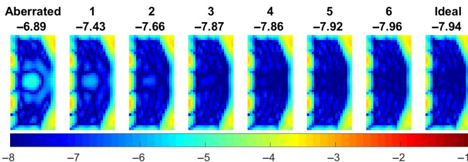
**Fig. 9** Evolution of the DF over the six iterations [seen in Fig. 10(b)] to converge from a degraded DF average contrast of  $10^{-6.90}$  with a  $10^{-5.0}$  magnitude speckle to the LDFC-corrected DF with  $10^{-7.94}$  average contrast. The ideal DF is shown in the final frame for reference. Scale is  $\log_{10}$  contrast.
