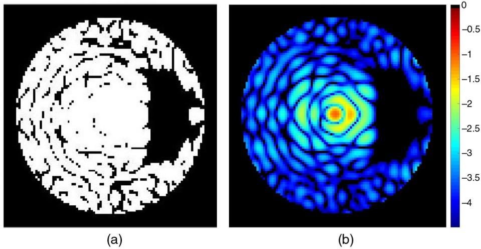
**Fig. 3** Images of the applied (a) BF pixel mask and (b) the  $\log_{10}$  masked reference image ( $I_{\text{ref},n}$ ). The binary mask passes only the pixels at or above the contrast threshold (shown in white). In this image, and for the following demonstrations, the contrast threshold was  $10^{-4.5}$ , and the outer diameter of the masked control area was set to be the control radius of the active area on the DM.
