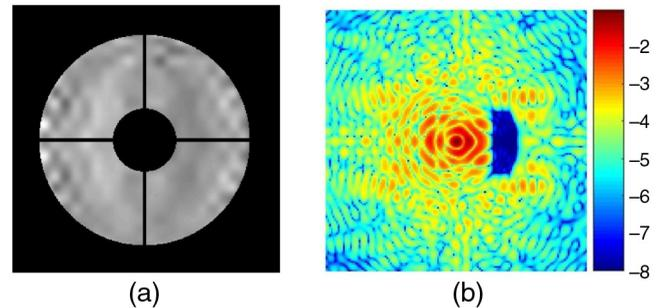
**Fig. 6** (a) Telescope pupil and standard implementation of EFC using a DM with 398 illuminated actuators to create (b) a  $3.5 \lambda/D \times 8.5 \lambda/D$  DF centered at  $6.75 \lambda/D$  from the center of the stellar PSF with  $10^{-7.94}$  average contrast.
