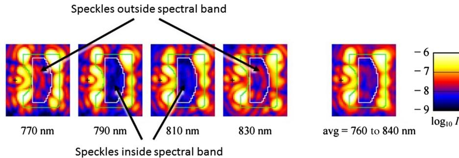
**Fig. 15** Spectral LDFC example: the  $7 \lambda/D \times 8 \lambda/D$  DF from JPL's HCIT created using a PIAA coronagraph. The DF is shown in four individual spectral channels: two channels within the control bandwidth and two out-of-band channels with speckles used to maintain the DF state within the control bandwidth. Also shown is the average DF over the full 10% bandwidth centered at  $\lambda = 800$  nm.<sup>20</sup>
