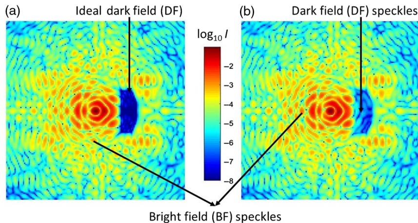
**Fig. 1** (a) Spatial LDFC:  $3.5 \lambda/D \times 8.5 \lambda/D$  DF created in simulation using conventional EFC. (b) Wavefront aberrations produce speckles in the BF and the DF, which degrade the DF. The change in intensity between (b) the aberrated BF and (a) the ideal BF is used to measure and cancel the speckles in the DF.
