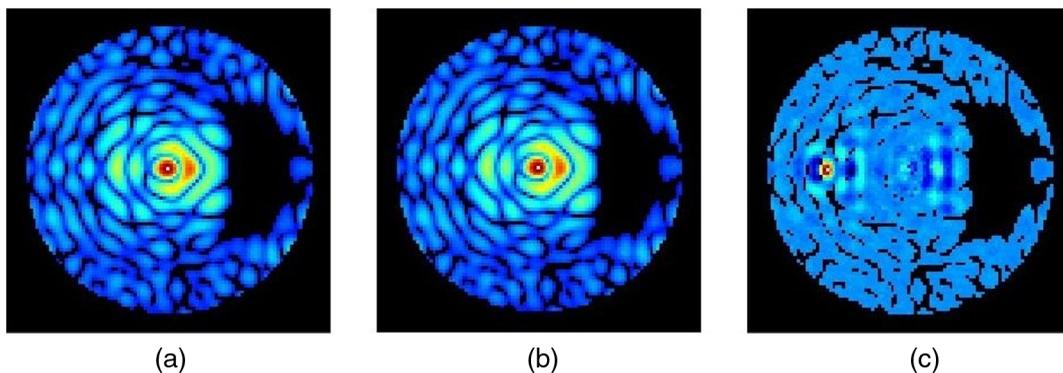
**Fig. 4** The BF pixels that are used in the (a) reference and (b) aberrated images to measure the (c) intensity change  $\Delta I_{t,n}$  that drives the spatial LDFC control loop to stabilize the DF. In all three images, the  $3.5 \lambda/D \times 8.5 \lambda/D$  DF can be seen to the right of the PSF core.
