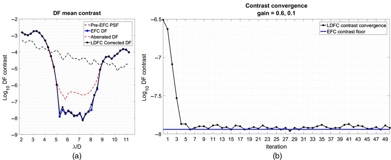
**Fig. 14** Performance of the spatial LDFC servo with a Kolmogorov phase perturbation. Gain = 0.6 until the DF contrast reached  $10^{-7.9}$ . The gain was lowered to 0.1 for the remaining iterations. (a) Average contrast across the full DF for the pre-EFC PSF, DF post-EFC (blue), DF post-EFC with injected speckle (red), and the corrected DF post-LDFC (black). (b) Average DF contrast (black) over 50 LDFC iterations showing convergence to the initial EFC contrast (blue) after six iterations.
