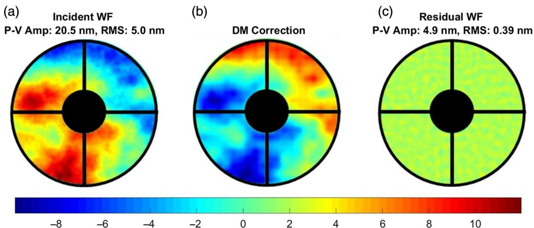
**Fig. 11** The injected Kolmogorov phase perturbation with (a) a P-V amplitude of 20.5 nm (RMS: 5 nm), (b) the DM response derived by LDFC, and (c) the final residual wavefront error (RMS: 0.39 nm) after six iterations. Scale is given in nm.
