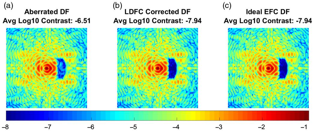
**Fig. 12** (a) The aberrated PSF with multiple speckles in the DF and average DF contrast of  $10^{-6.51}$ , (b) the final LDFC-corrected DF with  $10^{-7.94}$  average DF contrast, and (c) the reference EFC-derived DF with  $10^{-7.94}$  average DF contrast. Scale is  $\log_{10}$  contrast.
