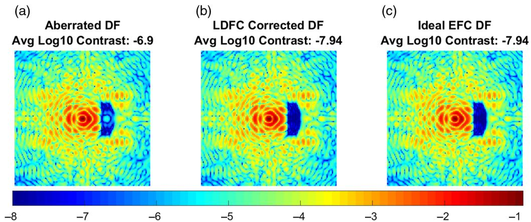
**Fig. 8** (a) The aberrated PSF with a single  $10^{-5.0}$  magnitude speckle in the DF with  $10^{-6.90}$  average contrast and a matching speckle in the BF, (b) the final LDFC-corrected DF with  $10^{-7.94}$  average DF contrast, and (c) the reference EFC-derived DF also with  $10^{-7.94}$  average DF contrast. Scale is  $\log_{10}$  contrast.
